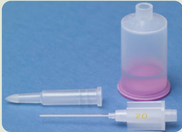
FIGURE 13-17 Parts of Unopette system used to dilute blood sample for WBC and platelet counts. Source: Delmar/Cengage Learning.
