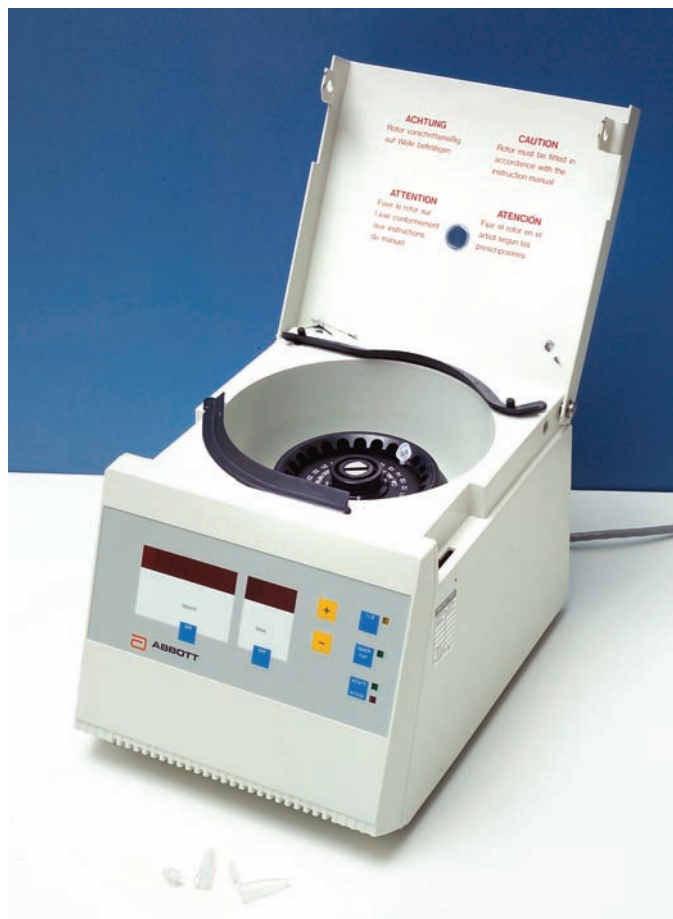
FIGURE 7-3 Microcentrifuge for small types of specimen containers. Source: Delmar/Cengage Learning.
