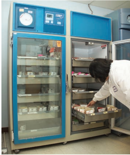
FIGURE 7-8 Blood bank refrigerator designed to store units of blood according to group and type, and special units for patients with unusual blood types or atypical antibodies. Source: Delmar/Cengage Learning.
