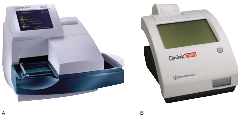
FIGURE 12-8 (A) The CLINITEK® 500 Urine Chemistry Analyzer is a semi-automated, benchtop analyzer that is capable of processing high volumes of samples; a urine chemistry dipstick may be processed every 7 seconds. (B) The Clinitek® Status is used for lower volume testing and handles one urine chemistry dipstick at a time. Source: Delmar/Cengage Learning.
