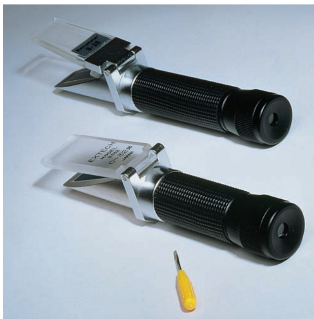
FIGURE 12-4 Refractometers operate by the bending of light waves by dissolved particles. Source: Delmar/Cengage Learning.
