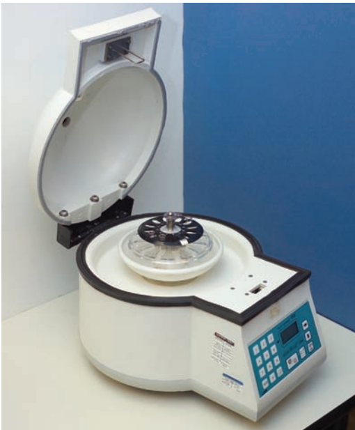
FIGURE 7-7 Serological centrifuge, used for preparing red blood cells for testing in blood banking procedures. Source: Delmar/Cengage Learning.
