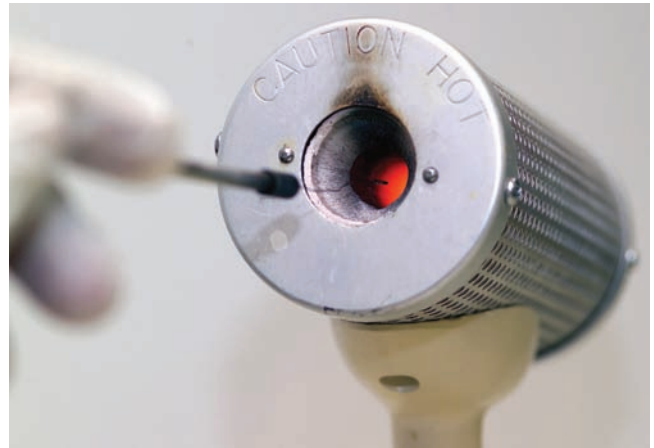
FIGURE 15-2 A bacterial incinerator, a work practice control, is used to avoid aerosols when an inoculating needle is sterilized. Source: Delmar/Cengage Learning.
