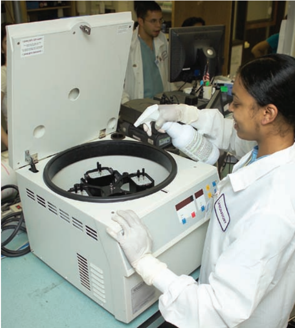
FIGURE 7-5 Disinfecting a clinical centrifuge. Source: Delmar/Cengage Learning.
