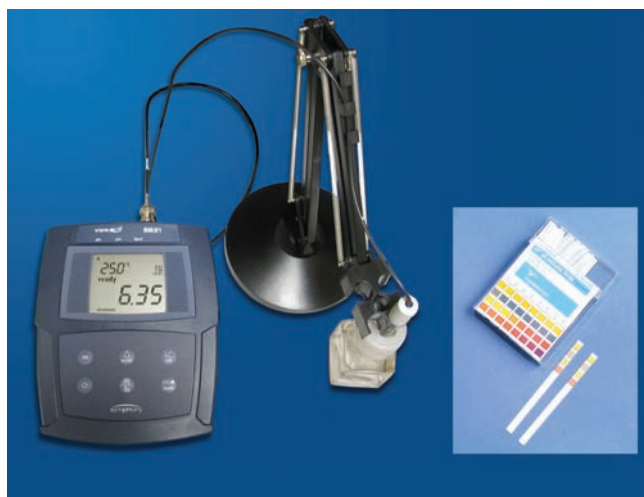
FIGURE 9-6 pH meter along with pH indicator strips used for basic screening tests for pH.
