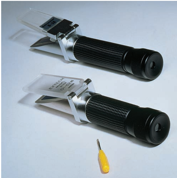
FIGURE 9-8 Refractometer that compares solutions with air. Source: Delmar/Cengage Learning.
