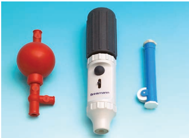
FIGURE 8-10 Pipetting aids for aspirating and dispelling solutions.
