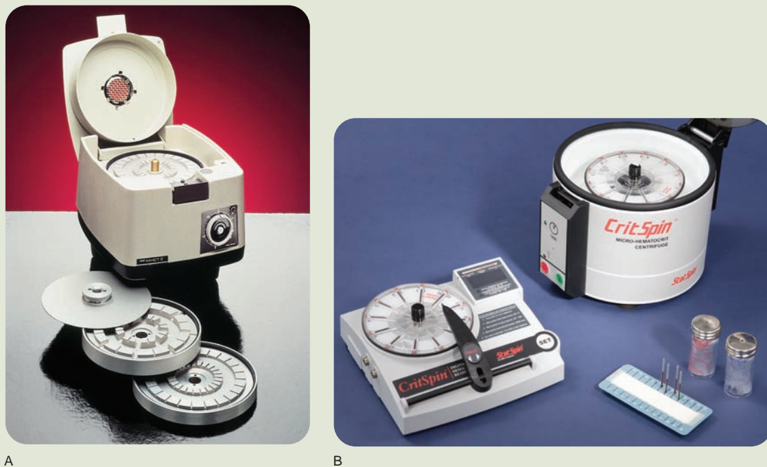
FIGURE 13-8 (A) Microhematocrit centrifuge with two sizes of centrifuge heads. (B) Crit-Spin centrifuge with microhematocrit reader and capillary tubes with sealant. Source: Delmar/Cengage Learning.
