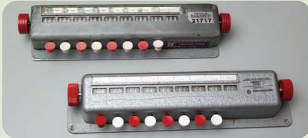
FIGURE 13-5 Differential white blood cell counter (manual) for determining percentages of the various types of white blood cells. Source: Delmar/Cengage Learning.
