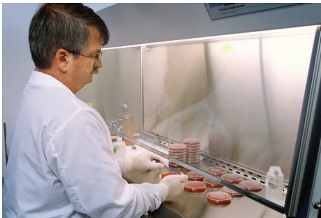
FIGURE 15-1 Biological safety cabinet for working with contagious organisms.
