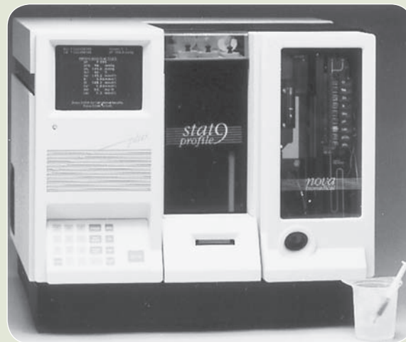
FIGURE 14-5 Nova CCX analyzer that uses ion-selective electrode technology for a variety of analyses. Source: Delmar/Cengage Learning.
