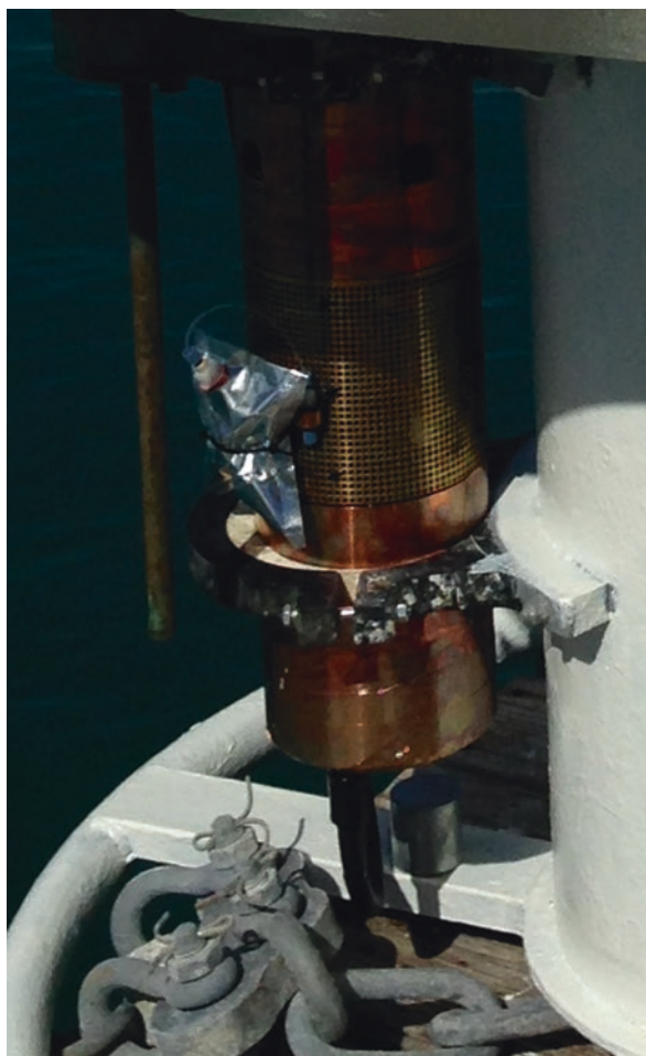
Fig. 2.14 Dye-based field pH meter installed on a data buoy
