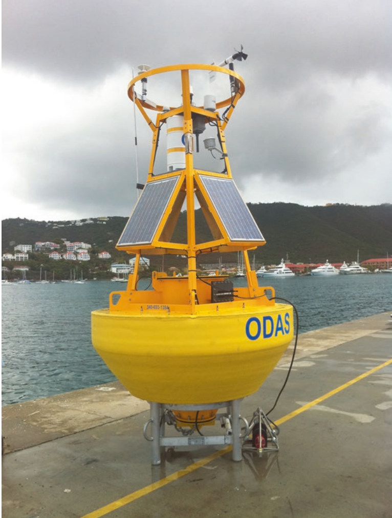
Fig. 3.2 ODAS buoy in preparation for deployment south of St. John, US Virgin Islands. Acoustic and rotor anemometer and meteorological instruments, in addition to GPS and communications antennae, are emplaced on the top railings and tower struts. An acoustic Doppler current profiler to be mounted integral to the mooring chain is enclosed in a stainless steel cage alongside the buoy base. A conductivity temperature/instrument is mounted horizontally on the right-hand base strut. The cylindrical instrument and battery well protrudes above and below the pan-shaped yellow buoyancy foam girdle. Solar photovoltaic panels provide electrical power
