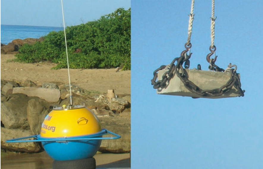
Fig. 3.3 Wave buoy and bottom mooring. Buoy to left, concrete anchor and chain to right
