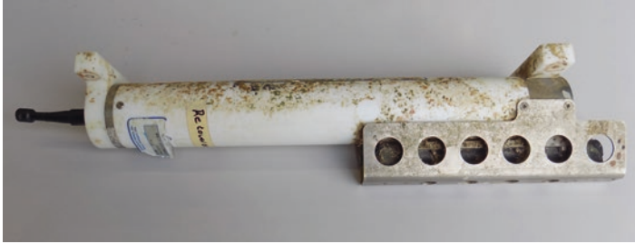
Fig. 2.13 Temperature/conductivity instrument. A cylindrical glass flow-through conductivity cell and a thermistor thermometer mounted externally on the cylindrical housing are protected by the perforated aluminum shield
