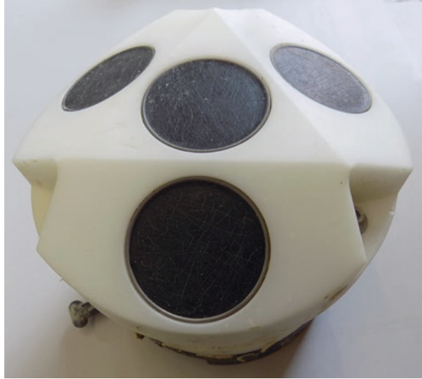
Fig. 2.9 Acoustic wave and current Doppler profiler. The central transducer follows the free surface yielding wave height while the lateral array tracks wave-induced orbital motion yielding wave direction. Additionally, the lateral array provides current velocity readings
