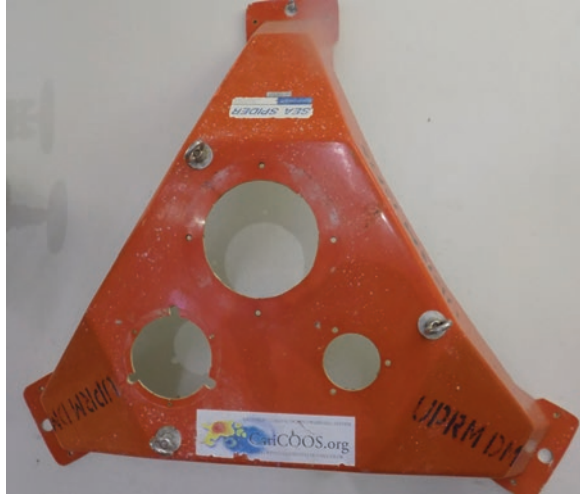
Fig. 3.5 Trawl resistant frame for instrument emplacement on the ocean bottom
