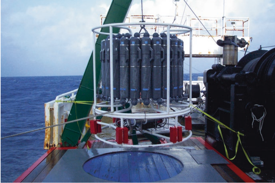
Fig. 3.6 Twenty-four bottle carousel fitted with 10 l bottles. A CTD equipped with chlorophyll, dissolved oxygen, and turbidity sensors is mounted in a stainless steel cage below the bottles. Red bricks are lead weights to facilitate deployment. The operating winch equipped with electromechanical cable is to the right of the carousel
