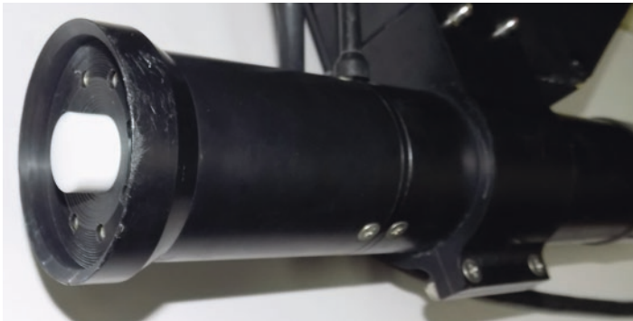
Fig. 2.12 Cosine collector quantum sensor (PAR meter)
