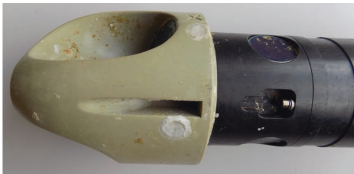
Fig. 2.3 Acoustic Doppler current profiler. One of three profiling transducers is visible in the head well. Two transducers of the three in the single depth array are visible mounted flush to the housing cylinder
