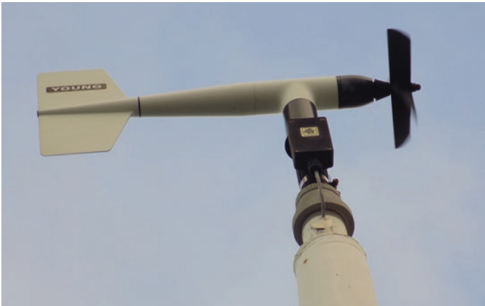
Fig. 2.10 Mechanical anemometer incorporating pivoting body, helicoidal rotor, and vertical tail vane
