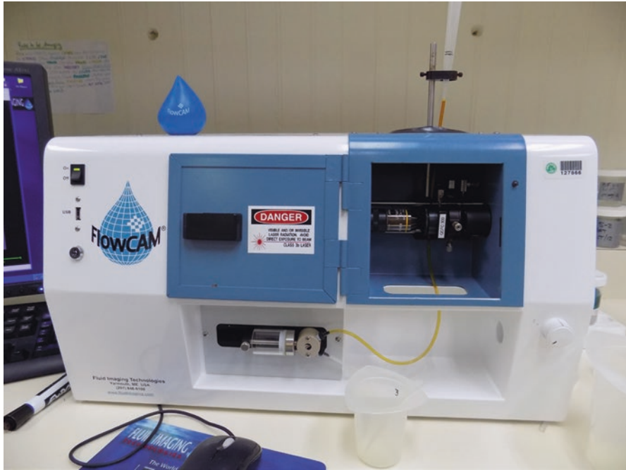
Fig. 2.18 Benchtop flow-through imaging and fluorescence instrument for phytoplankton characterization
