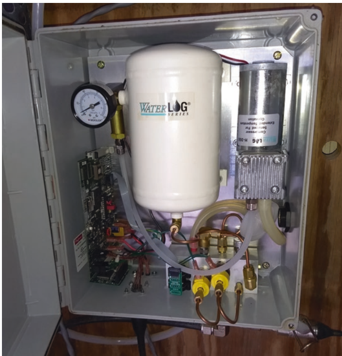
Fig. 2.8 Pneumatic system for bubbler tide gauge. Piston compressor on right, pressure vessel on left, valve body at bottom
