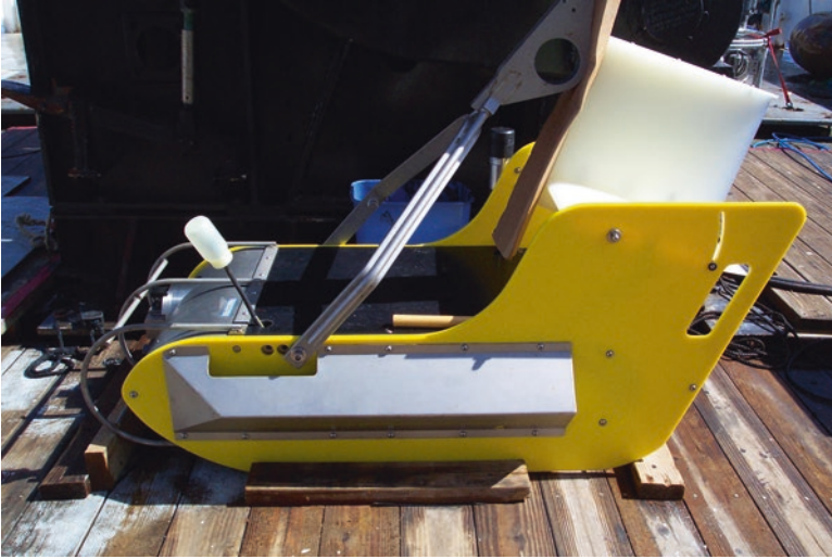
Fig. 3.7 Towed undulating vehicle. The vehicle pictured is fitted with CTD, chlorophyll fluorometer, and dissolved oxygen optode
