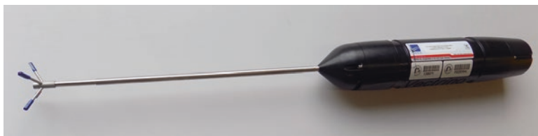
Fig. 2.2 Acoustic velocimeter for single-point current measurement. The instrument measures current velocity in a small volume of water at the focus point forward of the transducer array
