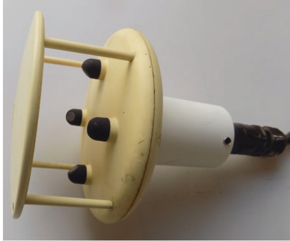
Fig. 2.11 Acoustic anemometer. Four ultrasonic transducers are visible
