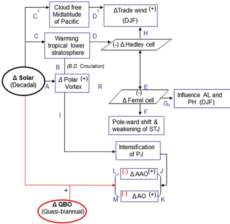
Fig. 11.8 Flow chart for stratosphere–troposphere coupling involving Sun and QBO (Roy 2014)
