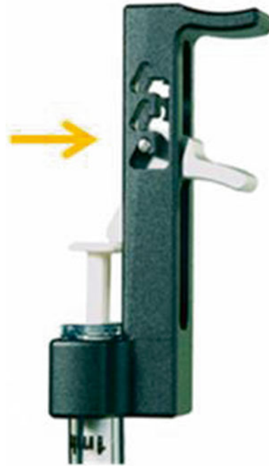
Fig. 6 Image of the syringe clip in the lowest position of Bioanalyzer System (Agilent Technologies)
