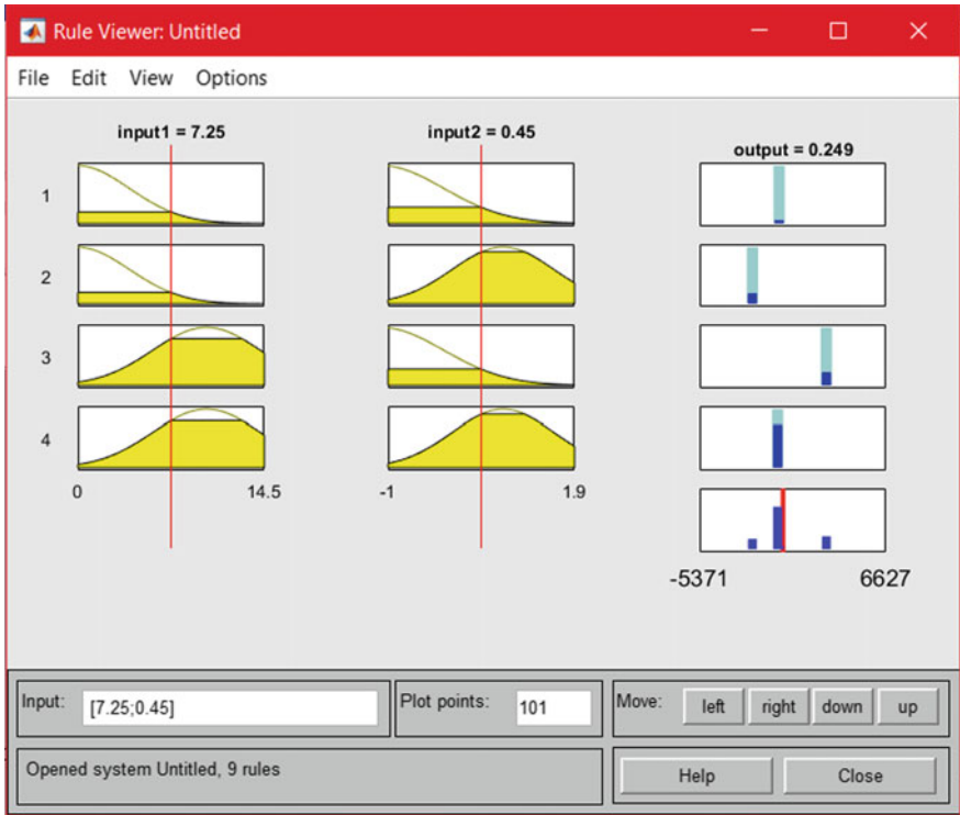
Fig. 5.30 Rules for type of MF Gaussian, output MF linear, grid partitioning, no. of epochs 40
