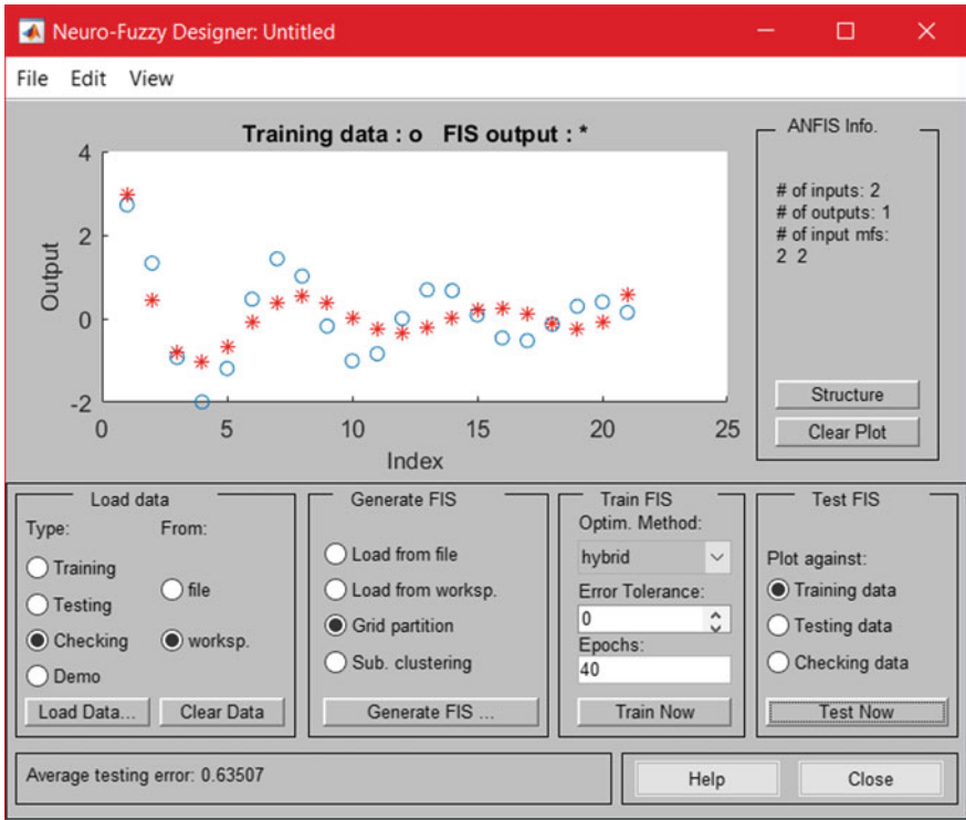
Fig. 5.27 Membership functions for inputs, type of MF Gaussian, output MF linear, grid partitioning, no. of epochs 40
