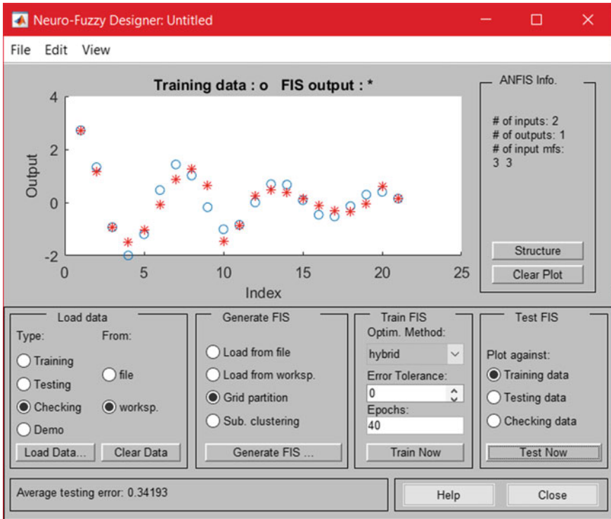
Fig. 5.29 ANFIS with 3 MFs for input (x1) and 3 MFs for input (x2) and MFs type triangle and linear MF output, after only one epoch training
