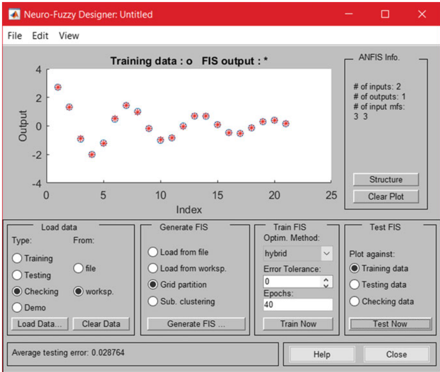
Fig. 5.28 Three membership functions for inputs, type of MF Gaussian, output MF linear, grid partitioning, no. of epochs 40
