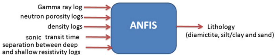
Fig. 6.42 Input/output of ANFIS lithology interpreter
