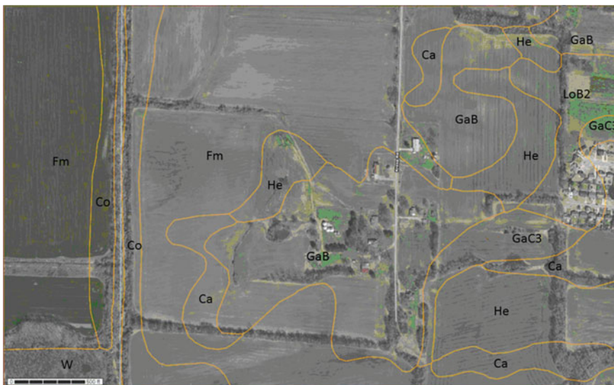
Fig. 5.24 Soil map of the test site (lines are the borders between soil types; Ca is Calloway silt loam, Co is Collins silt loam, Fm is Falaya silt loam, GaB is Grenada silt loam, GaC3 is Grenada silt loam, He is Henry silt loam, and LoB2 is Loring silt loam) (Web soil survey 2014)
