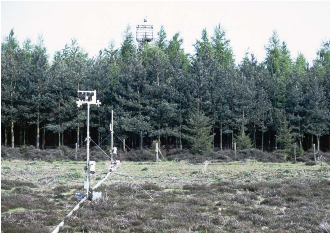
Fig. 5.6 The Berners Heath–forest interface experiment showing two of the eight Mk1 HYDRAs on a transect between the heath and the forest. (Source: Reproduced with permission of CEH.)
