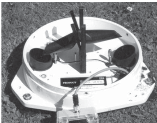
Fig. 2.12 Tipping bucket rain gauge (showing the interior). (Source: Reproduced with permission of Ian Strangeways.)
