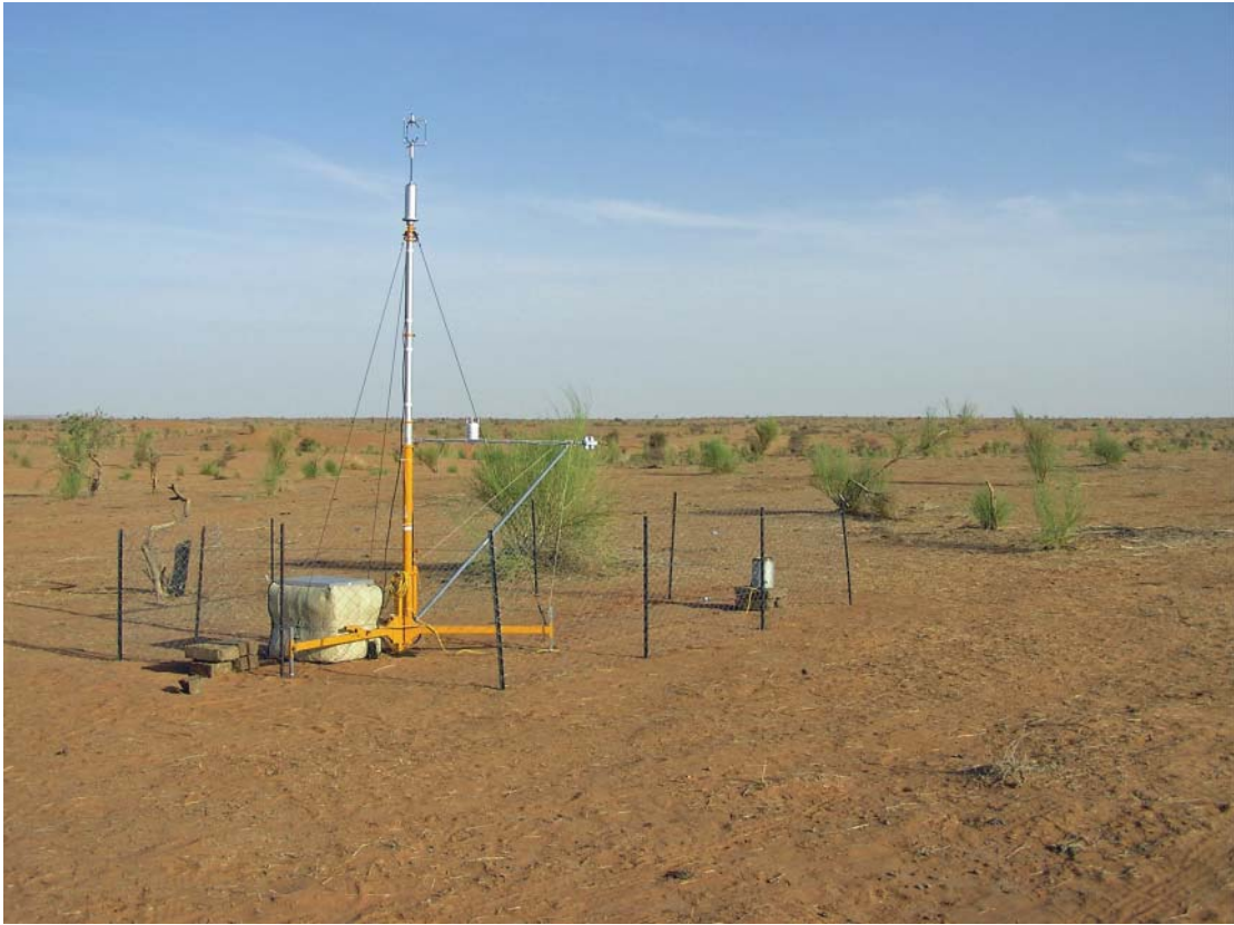
Fig. 5.19 The combined AWS/flux system at the desert margin site at Bamba. (Source: Reproduced with permission of Colin Lloyd.)
