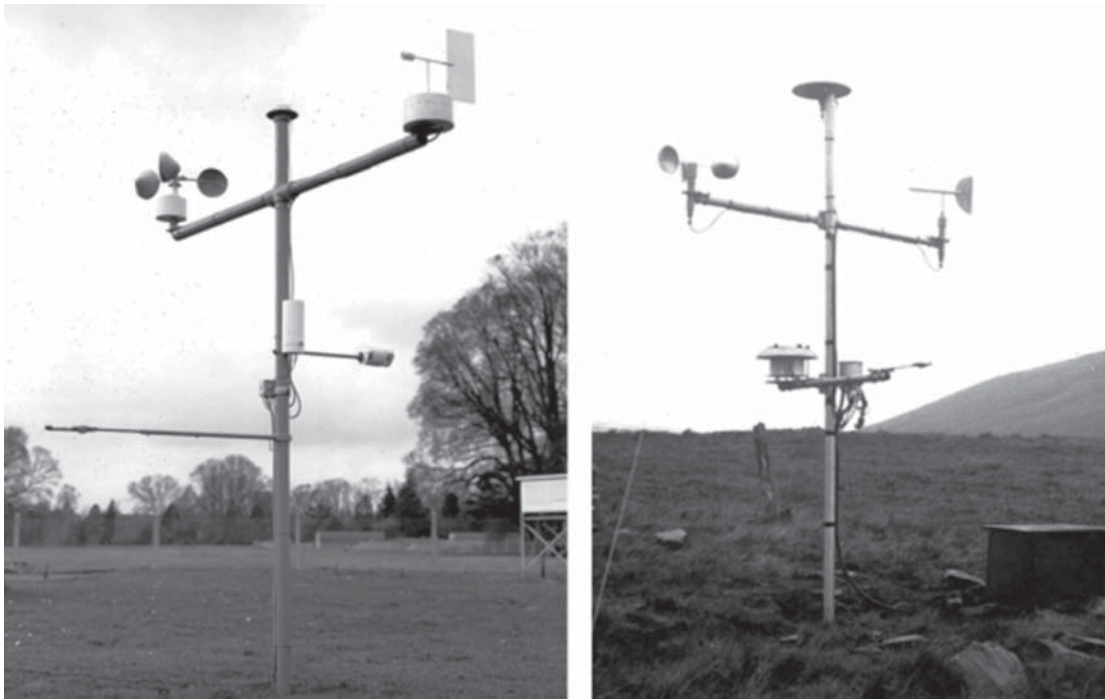
Fig. 2.13 Automatic Weather Stations: Left : Early prototype developed at IH in the late 1960s. One of the first modern AWSs. Right : Didcot Instruments production model – still in use. (Source: Reproduced with permission of Ian Strangeways.)
