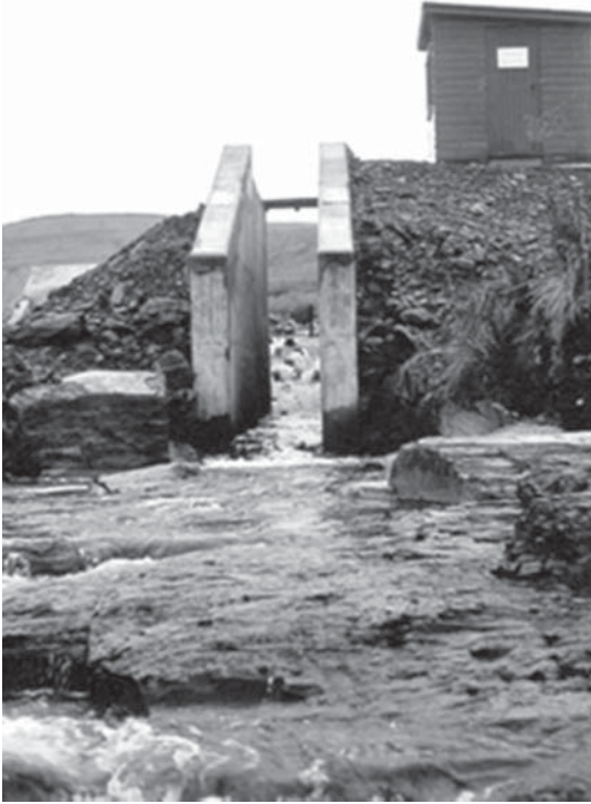
Fig. 2.17 Steep stream flume at Plynlimon. (Source: Reproduced with permission of CEH.)
