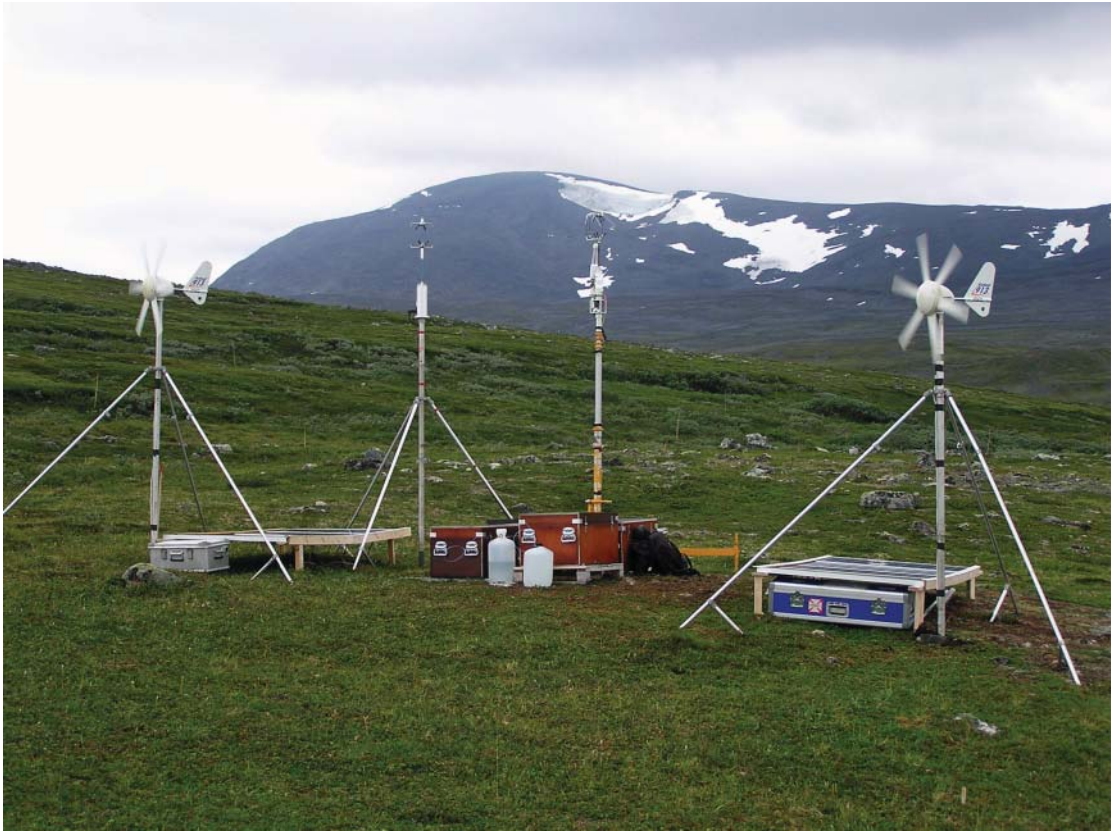
Fig. 5.18 Mk4 and Solent R3/Licor 7500 flux systems, wind generators and horizontal solar panels at the upland tundra site near Abisko, northern Sweden. (Source: Reproduced with permission of Colin Lloyd.)
