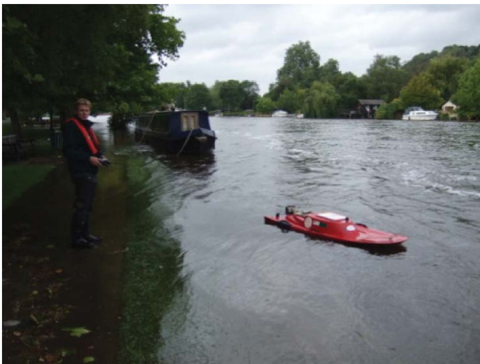
Fig. 11.11 Acoustic Doppler Current Profiler (ADCP) being deployed on the River Thames (Source: Reproduced with permission of CEH.)
