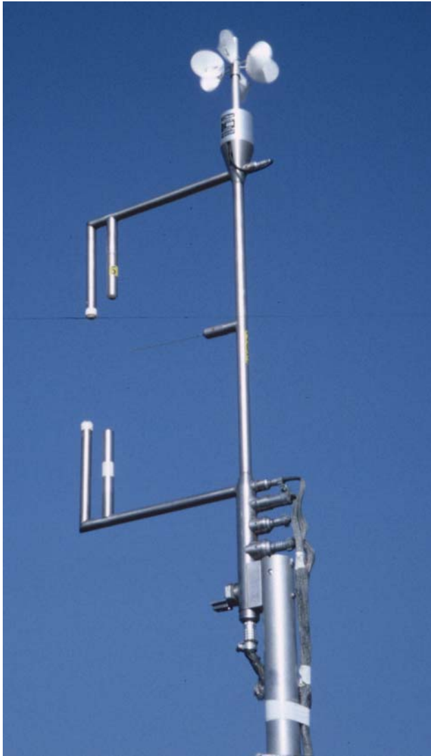
Fig. 5.12 The Mk2 HYDRA eddy correlation instrument. (Source: Reproduced with permission of John Gash.)
