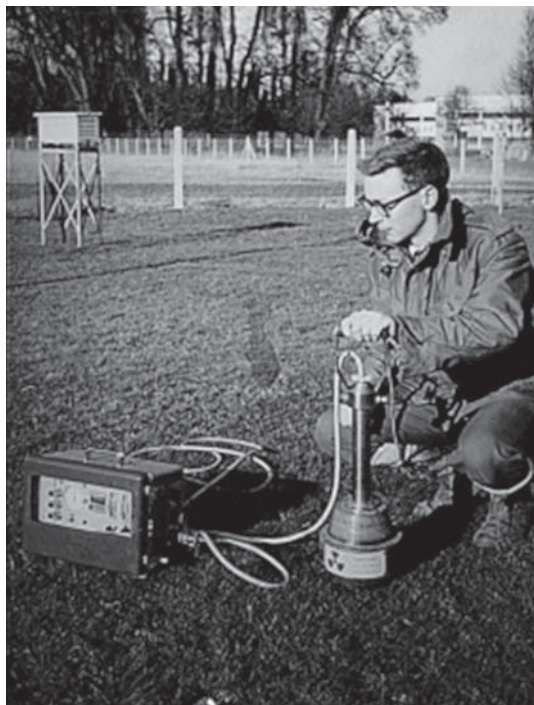
Fig. 2.18 Neutron probe 1 the Danbridge equipment showing scaler and transport shield. (Source: Reproduced with permission of CEH.)
