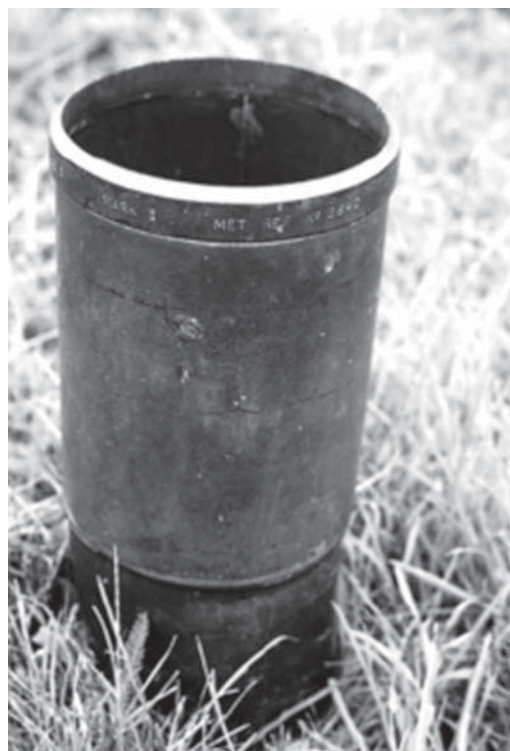
Fig. 2.6 The UK standard five-inch manual raingauge. (Source: Reproduced with permission of Ian Strangeways.)
