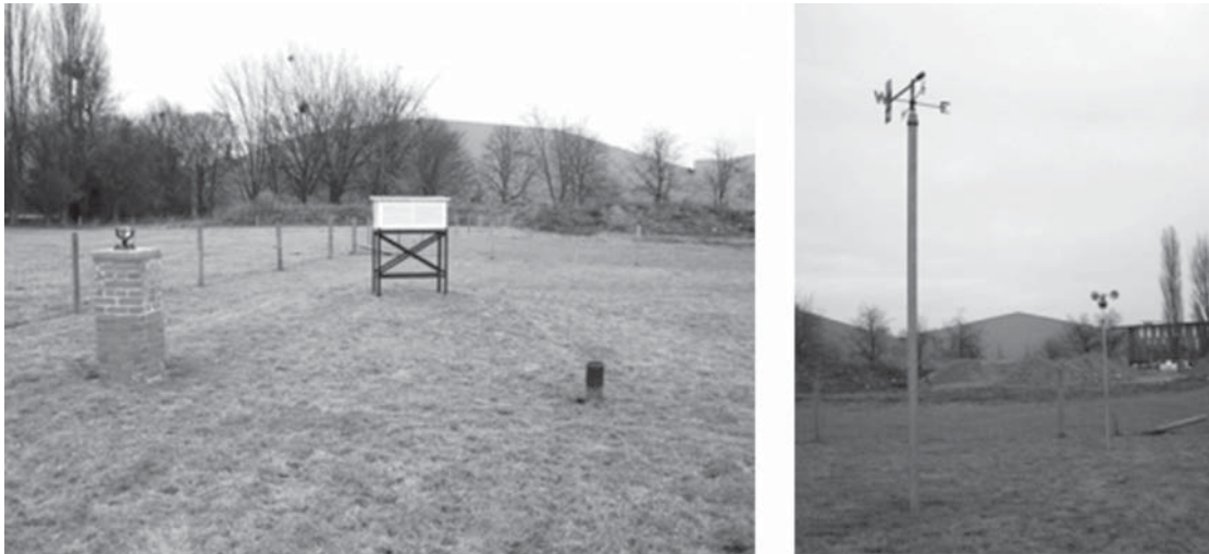
Fig. 2.4 A typical traditional Met Site. From left to right: Campbell-Stokes Sunshine recorder, Stevenson screen containing thermometers for recording maximum and minimum air temperature and 'wet and dry bulb' thermometers for measuring relative humidity, with a five inch manual raingauge. In right photo are the wind direction and windspeed sensors. (Source: Reproduced with permission of Ian Strangeways.)
