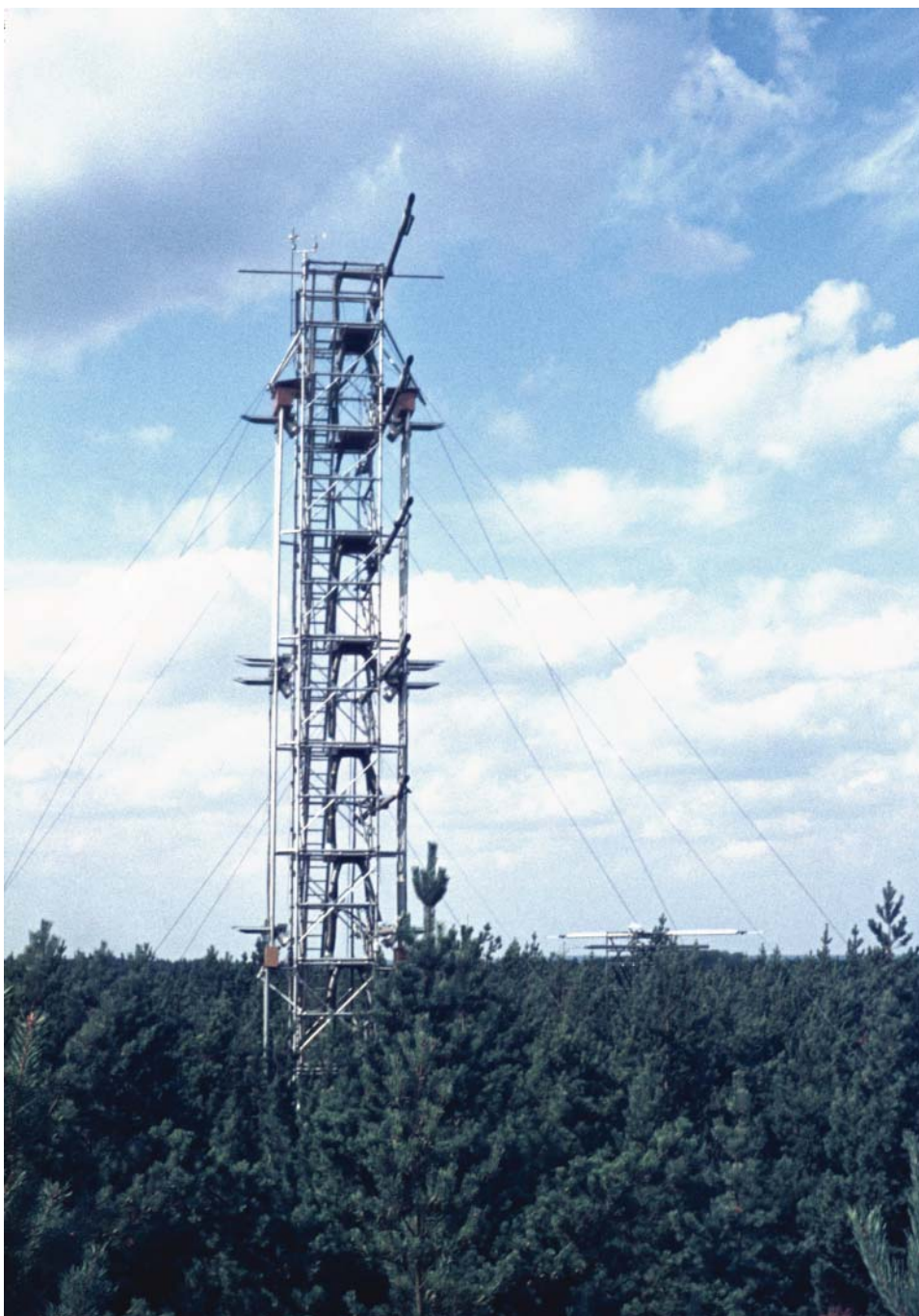
Fig. 5.3 Two TIS Systems to account for all wind directions. (Source: Reproduced with permission of CEH.)
