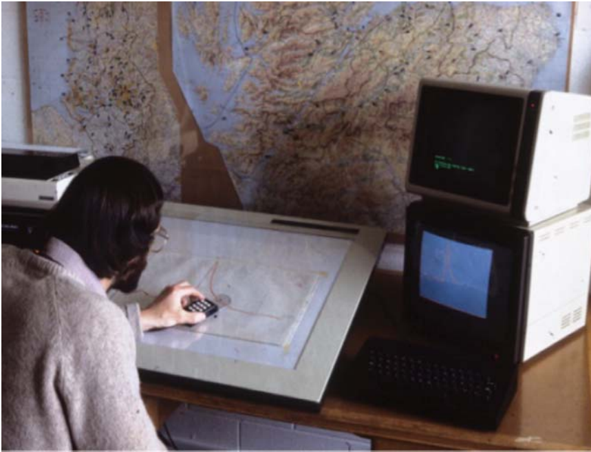
Fig. 11.4 Digitising a river level hydrograph. (Photo NRFA.) (Source: Reproduced with permission of CEH.)
