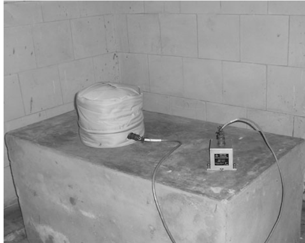
Fig. 2.3 BB and SMA installed on seismic pillar embedded to hard ground/rock at field station
