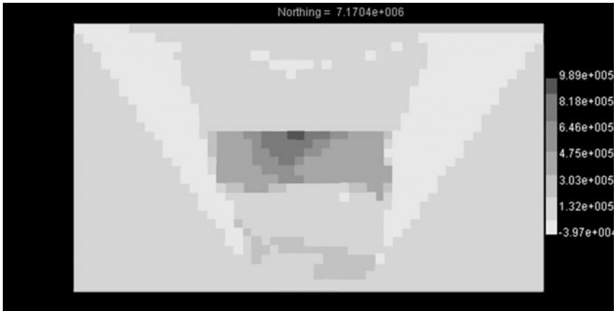
Fig. 1 Kriged block values for a vertical slice through our example pit
