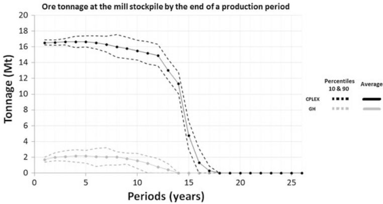
Fig. 3 Expected ore tonnage at the mill stockpile and related risk profiles, using CPLEX (black) and GH (gray) to generate initial solutions
