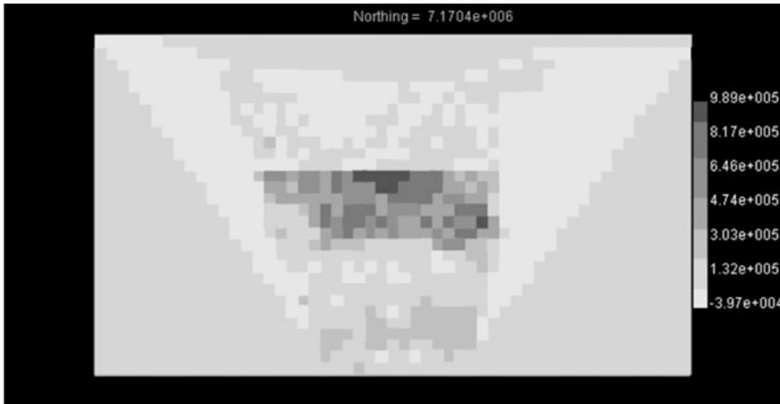
Fig. 5 Conditional simulation block values for a vertical slice through our example pit. This simulation has the lowest total block value
