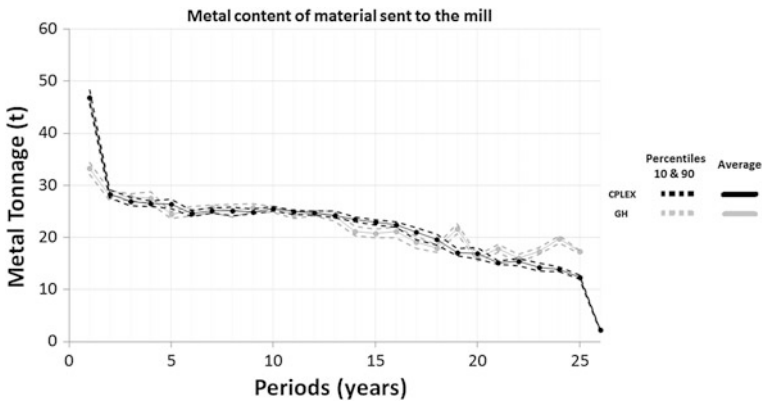
Fig. 4 Expected metal input to the mill and related risk profiles, using CPLEX (black) and GH (gray) to generate initial solutions
