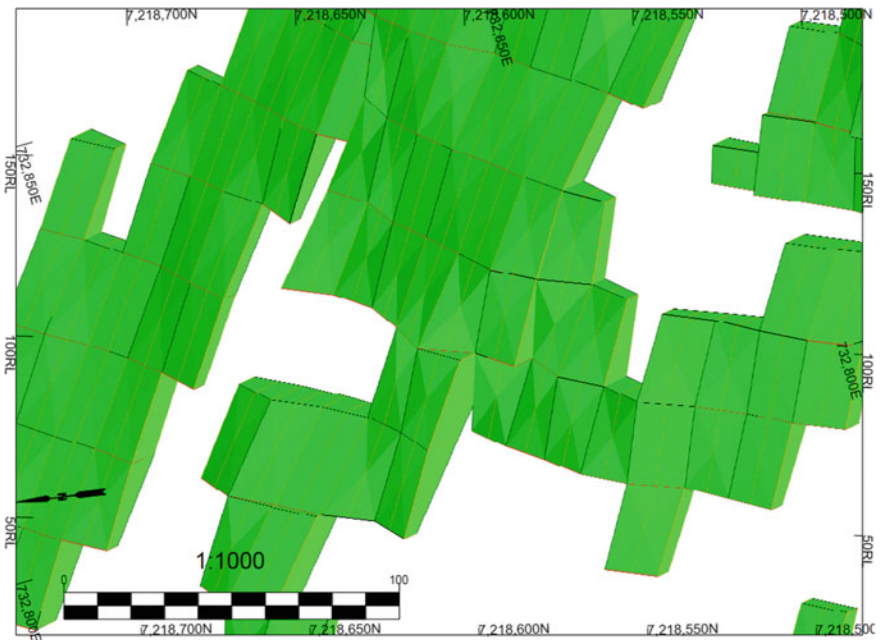
Fig. 4 Example AMS stope optimiser stope solids output in Deswik.CAD
