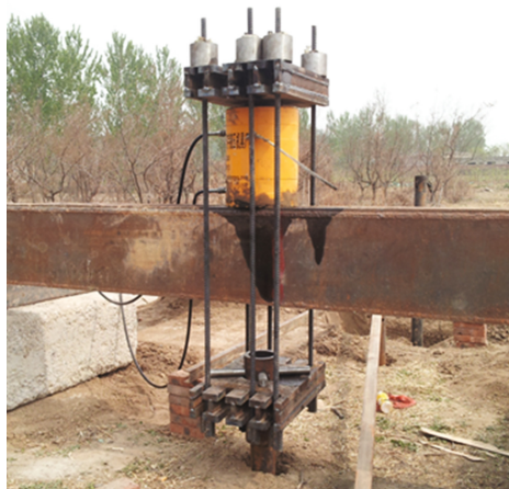
Fig. 3. Axial tension test setup
