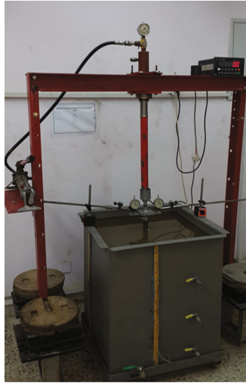
Plate 1. Loading frame and soil container
