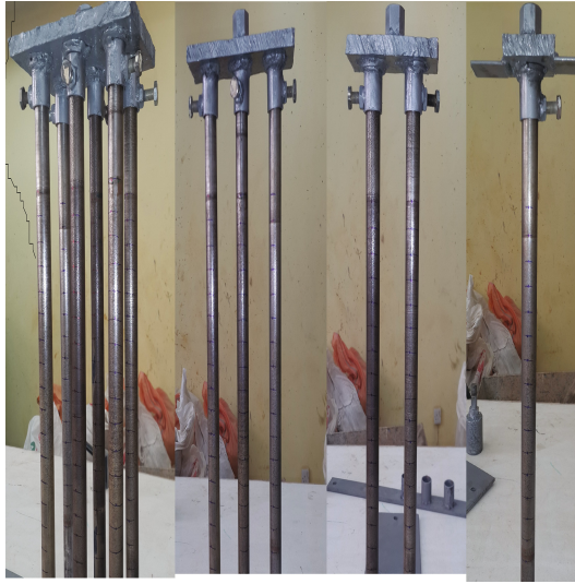
Plate 2. Pipe pile models with different configurations with fixing rings
