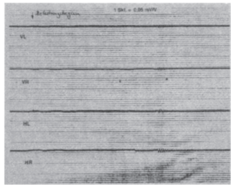
Fig. 6b. Force readings of device B (arrow indicates start of three-point bending).
