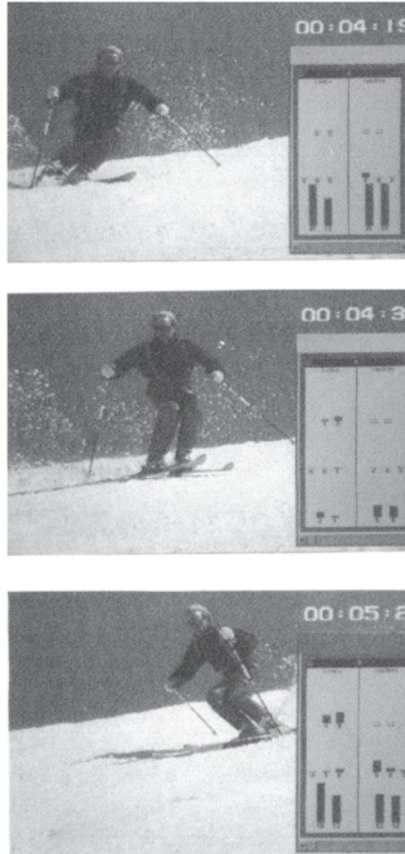
Fig. 11. Characteristic timing of the heel pressure during parallel short turns.
