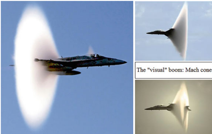
Fig. 7.13 The “visual” boom accompanying the sonic boom that appears when a supersonic aircraft exceeds the speed of sound. This image clearly exhibits the Mach cone in mechanics.
