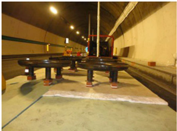
Fig. 3.21 Positioning of the fuel pans on the bricks
