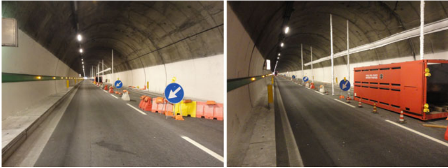
Fig. 3.17 Preparation of the accident scenario with the Morgex North tunnel open to traffic
