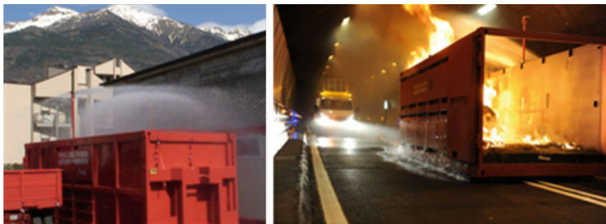
Fig. 3.3 Roll-off container used for the real-scale fire test
