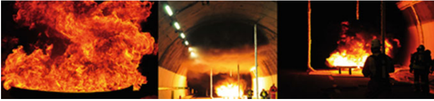
Fig. 4.1 Fire pictures: single pan fire ( left ), initial smoke back-layering ( center ) and firefighters ensuring safety during the experimental activity ( right )
