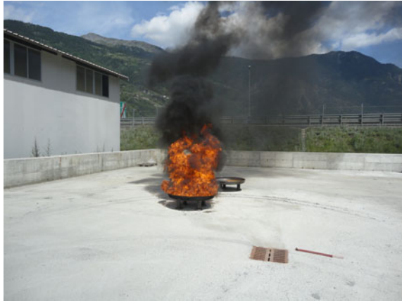
Fig. 3.7 Preliminary fire test using 20 L of diesel fuel
