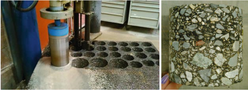
Fig. 5. Test specimen, left: slab for coring, right: cut 2 layer specimen
