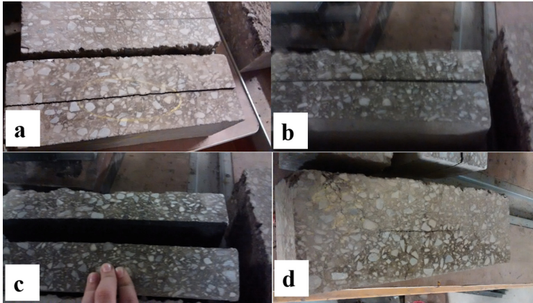
Fig. 11. Asphalt slabs disconnect at the bond line prior to test.
