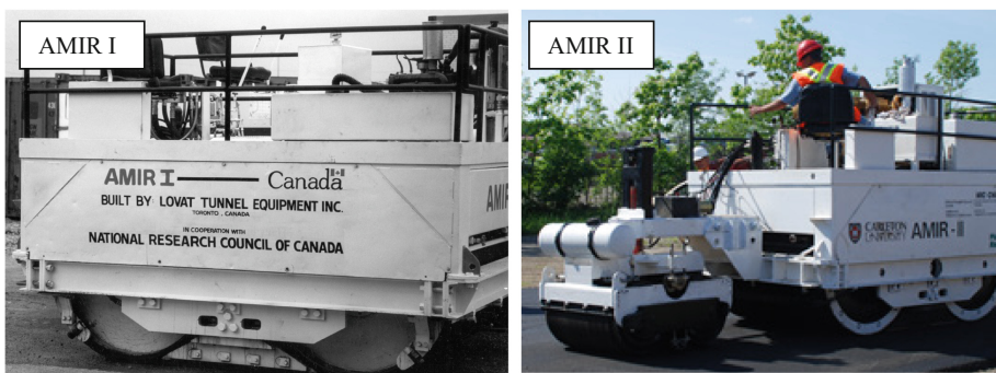
Fig. 2. The Asphalt Multi Integrated Roller (AMIR)
