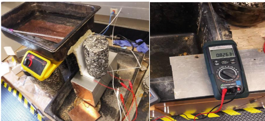
Fig. 8. Laboratory test setup of the prototype and power measuring device
