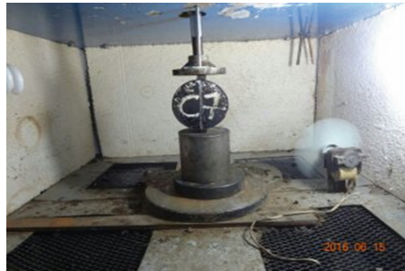
Fig. 3. Repeated indirect tensile test
