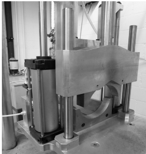
Fig. 1. LPDS static testing device
