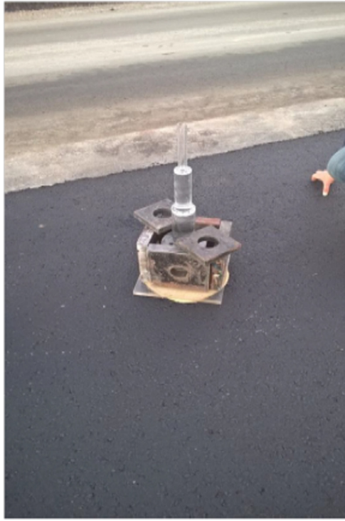
Fig. 9. Field measurement of permeability
