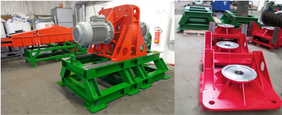
Fig. 1. High-speed disintegrator used within the experiments described by this paper (left) spreader annulus of rotors for placing of milling elements)
