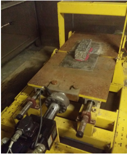
Fig. 1. Specially designed testing table, for DTT on asphalt concrete
