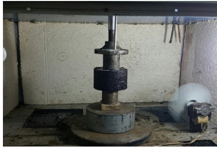
Fig. 4. Repeated punching shear test
