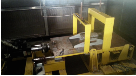
Fig. 2. Specially designed testing table, for DTT on asphalt concrete
