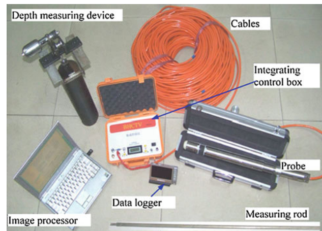
Fig. 1 The basic components of a typical borehole digital optical camera system. Note the photo of the components may change in case of the different borehole digital optical camera system
