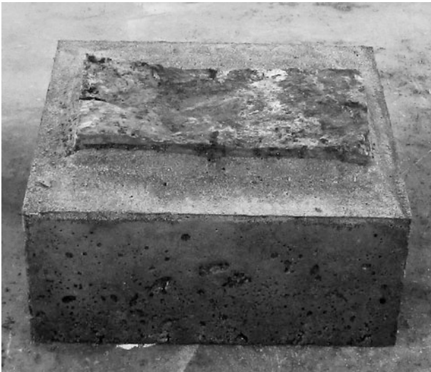
Fig. 3 Encapsulate lower half of a rectangular shaped test specimen
