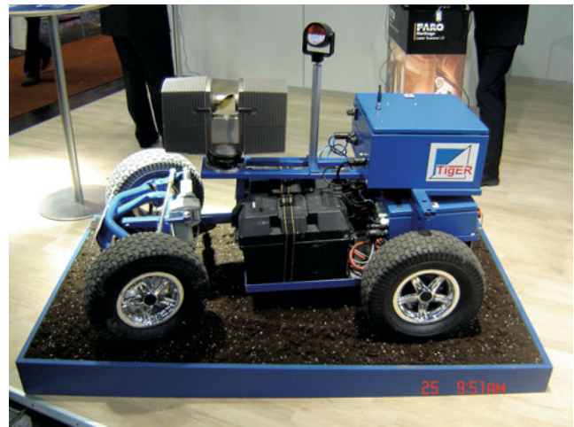
Fig. 4 A prototype of remote-control scanning system developed by Faro ( www.faro.com )
