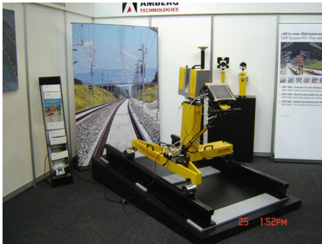
Fig. 5 Amberg GRP scanning system developed for railway scanning ( www.amberg.com )
