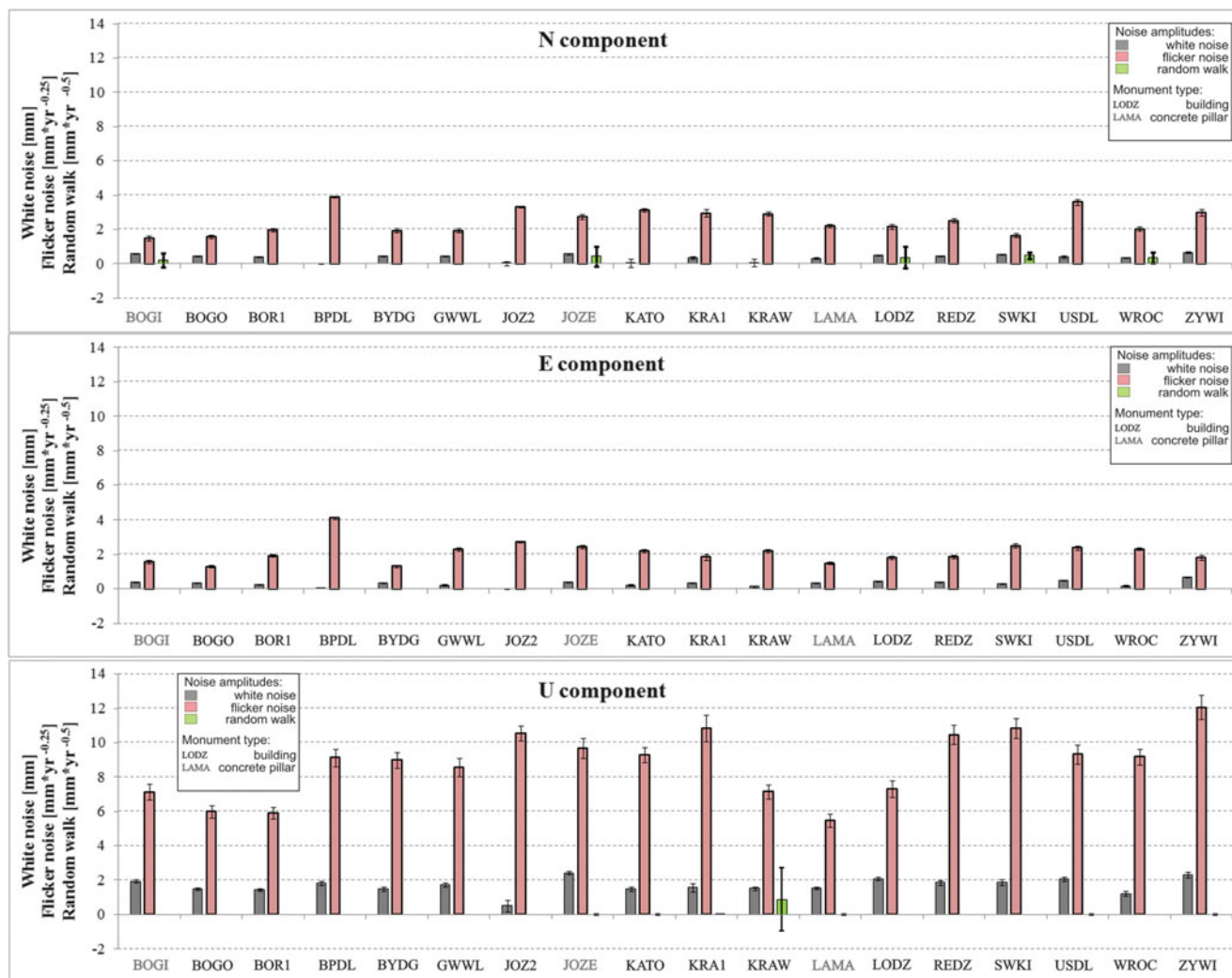
Fig. 4 Amplitudes of white noise (grey), flicker noise (pink) and random walk (green) for North (top), East (middle) and the Up (bottom) components obtained with the MLE method. For each of these amplitudes a 1-sigma error bar was added. Different types of
