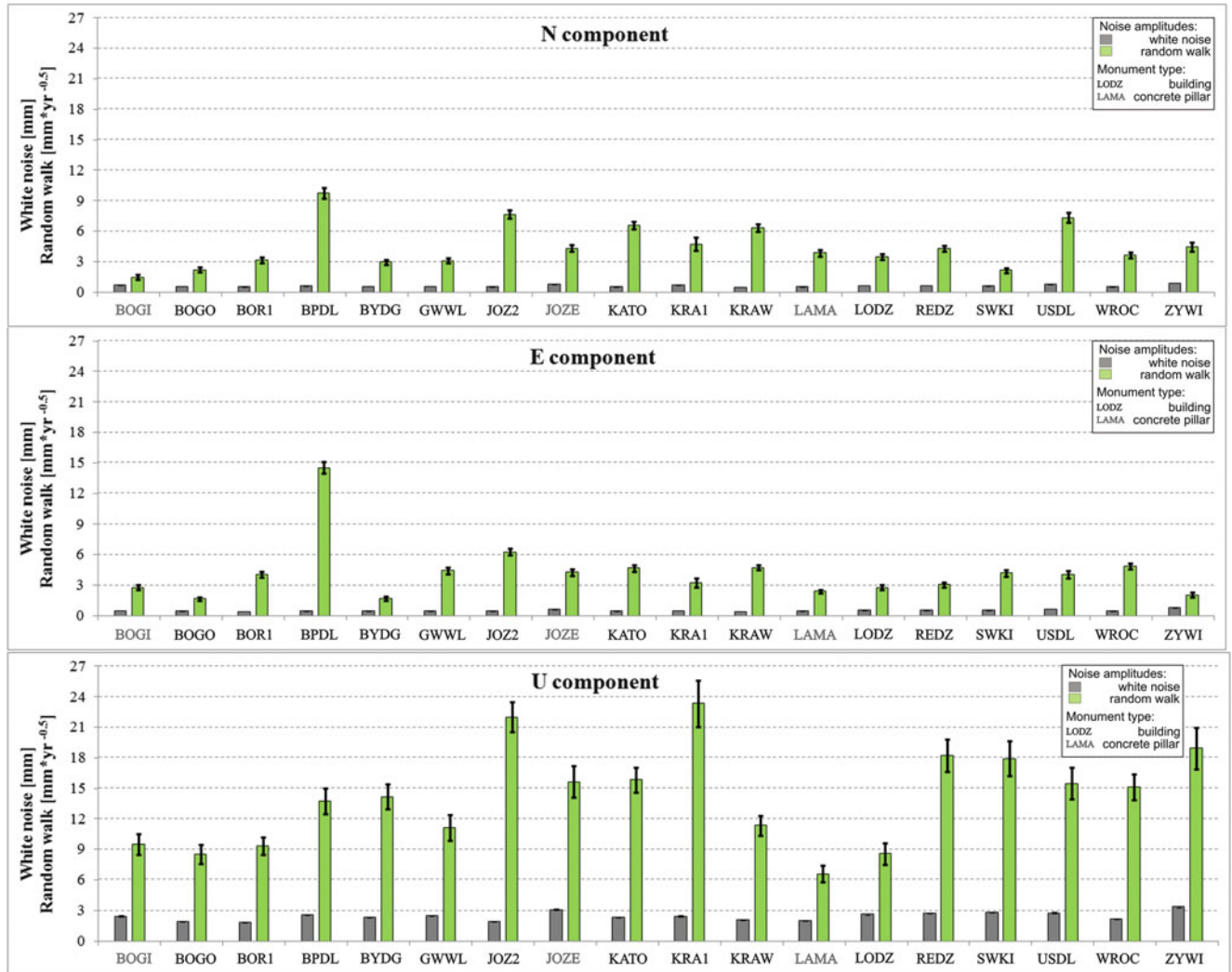
Fig. 6 Amplitudes of white ( grey ) and random-walk ( green ) noise for Polish EPN stations obtained with the MLE method with the assumption of WH and RW noise only. The plots are presented for North ( top ), East ( middle ) and Up ( bottom ) components. The 1-sigma error bars were added to each of amplitude
