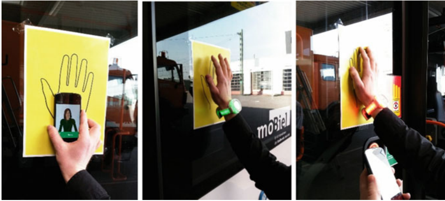
Fig. 9.2 Yellow plates equipped with RFID tags to identify a bus ( left using to NFC equipped smartphone to read the tag; middle special smartwatch with RFID reader showing a “right” bus; right special smartwatch with RFID reader showing a “wrong” bus)
