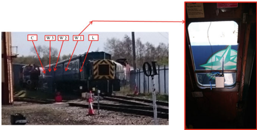
Fig. 6.5 Set-up of SPARTACUS system on testing train
