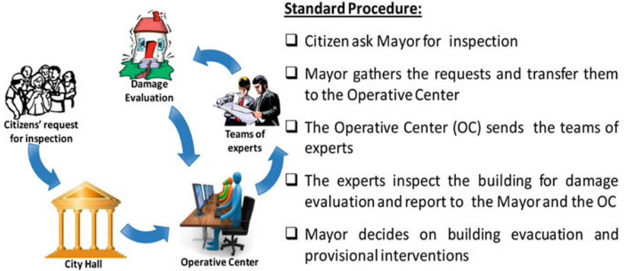
Fig. 8.43 Standard damage assessment
