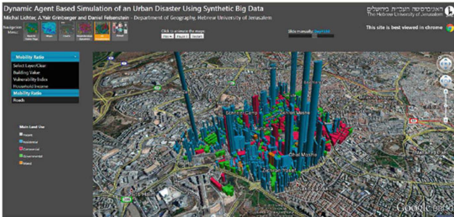
Fig. 14.34 3D visualization with Google Earth APIs as platform (The height of the columns represents the value of the variable selected on the left-hand menu. The color refers to the different type of structures)
