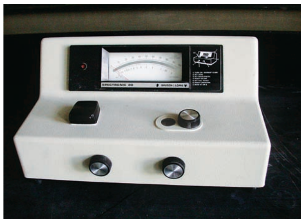
A spectrophotometer is an instrument that measures the amount of light that passes through a specimen. (Department of Biological Science, University of Manitoba)
