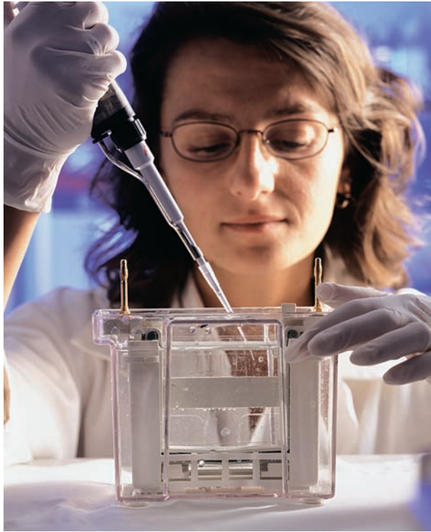
Polyacrylamide gel electrophoresis utilizes vertical apparatuses, and buffer tanks have contact only with the top and the bottom portion of the gel. (Mauro Fermariello/Photo Researchers, Inc.)
