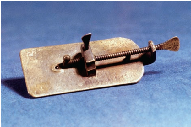
Leeuwenhoek's microscopes, such as the one shown here, contained a single lens that he ground himself and could obtain magnifications of up to 300 \times . (HIP/Art Resource, NY)
