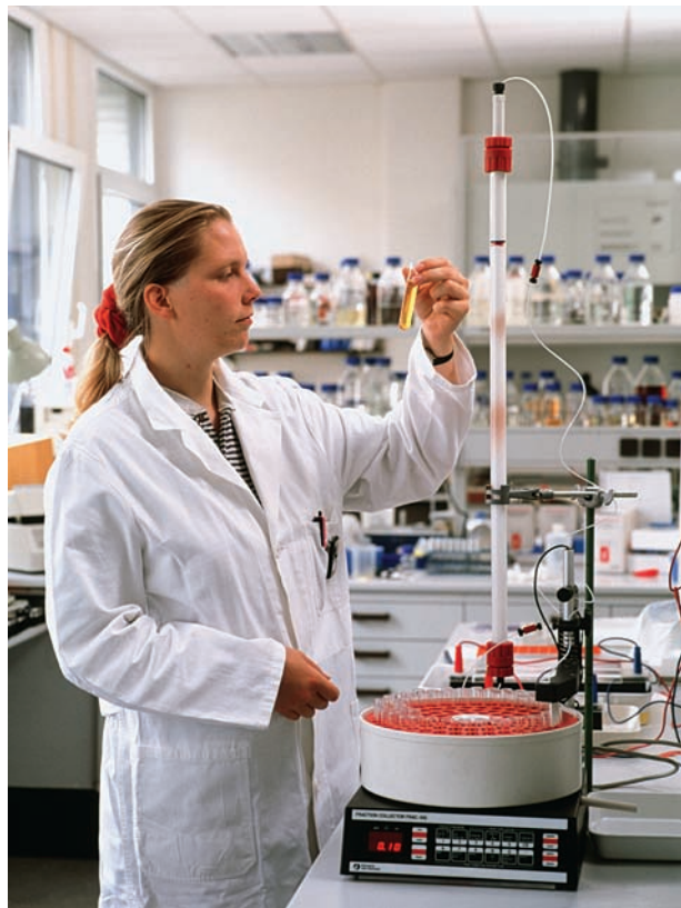
In column chromatography, a liquid mobile phase travels through a column packed with a material that retains mixture components to different degrees. (Maximilian Stock Ltd./Photo Researchers, Inc.)
