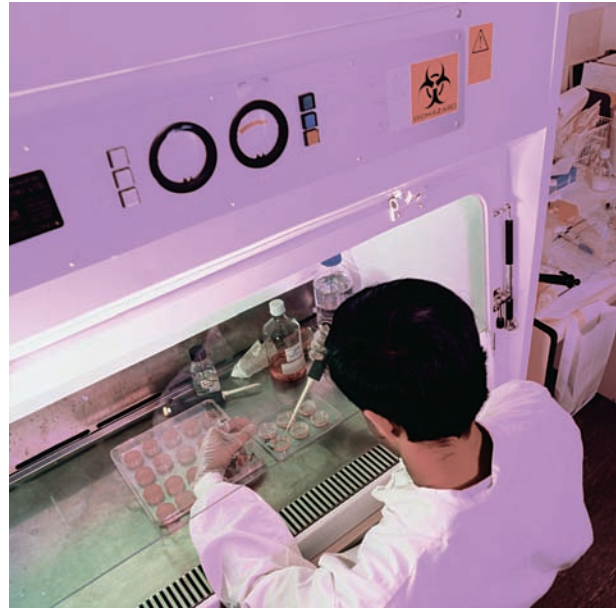
Handling and treating cell and tissue cultures within a laminar flow hood reduce contamination. (James King-Holmes/Photo Researchers, Inc.)
