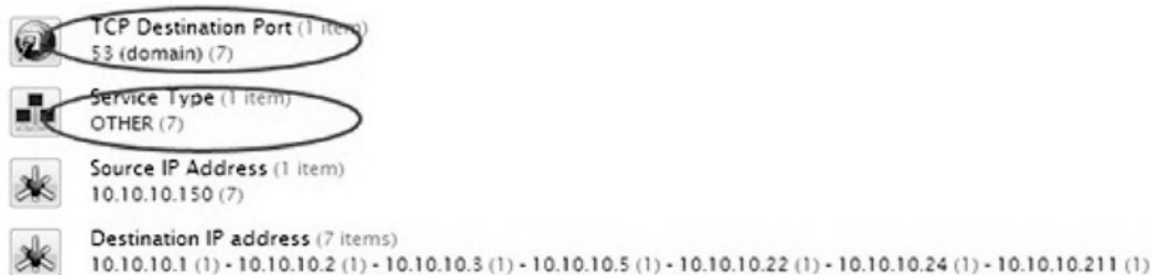
Fig. 7.15 Nonstandard network traffic on port 53
