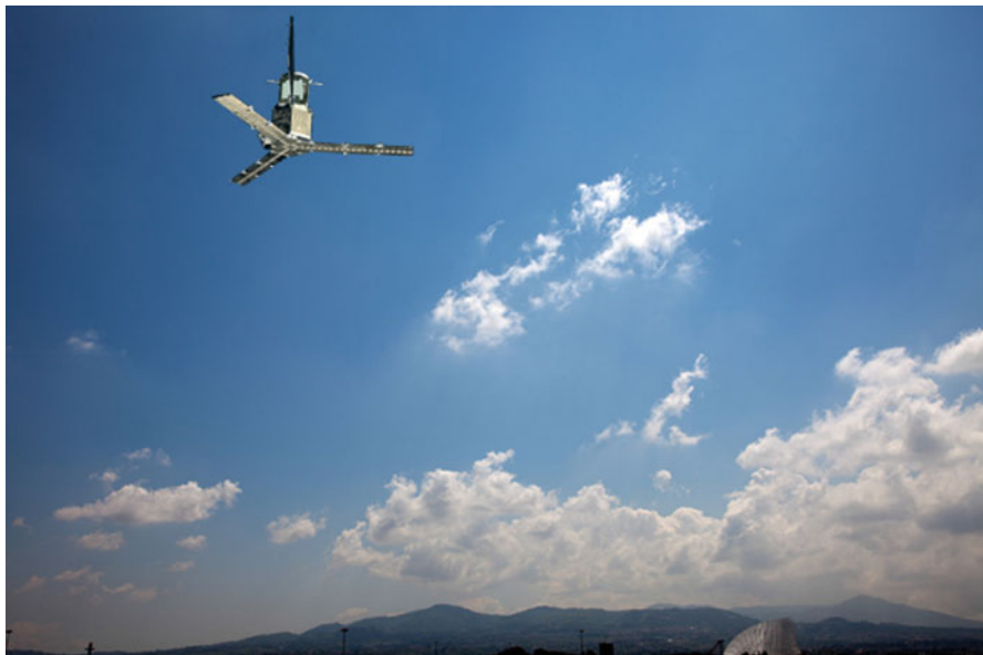
Fig. 11.11 SMOS, European space borne interferometric-antenna L-band radiometer; the three elongated panels form the two-dimensional array interferometer (Credit: satellite image, ESA; artwork, A. Perrone, Tor Vergata University Earth Observation Laboratory)
