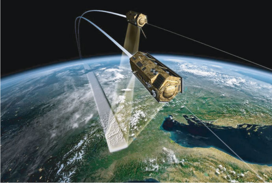
Fig. 12.27 The TanDEM-X Mission, which has operated since 12 October 2010, acquires interferometric image pairs simultaneously from two satellites in quasi-monostatic configuration (Credit: ©2010 DLR)
