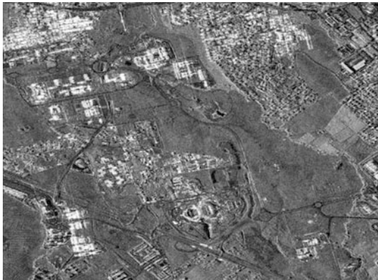
Fig. 10.24 Single-polarization ( \sigma_{hh}^0 ) metric-resolution COSMO-SkyMed image of part of Tor Vergata University campus, Rome, Italy; light grey corresponds to high values of \sigma^0 , dark to low (Credit: data, © ASI, 2010; processing, C. Pratola, Tor Vergata Earth Observation Laboratory)
