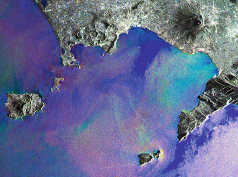
Fig. 14.52 ENVISAT ASAR RGB multi-temporal C-band image of the Gulf of Naples: coloring denotes changes of surface roughness essentially due to different wind speed fields on the dates of acquisition (Data credit: ESA; processing and image production, C. Solimini)
