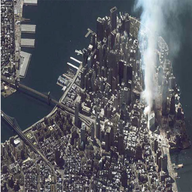
Fig. 12.3 Optical image of Manhattan taken on 12 September 2001: the effect of the elevation in moving the high pixels away from the satellite ground track is dramatically highlighted especially by the taller buildings and by the smoke plume (Credit: Space Imaging)
