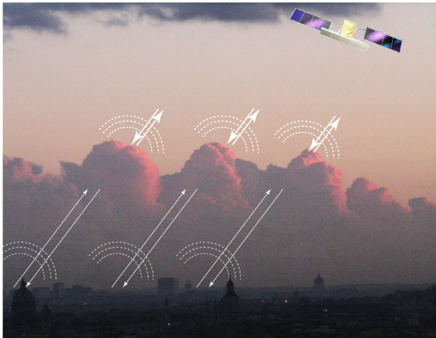
Fig. 10.13 Sketch of radar observation of the surface through clouds, with representation of scattering from convective cells (COSMO-SkyMed, © ASI; artwork by A. Perrone)
