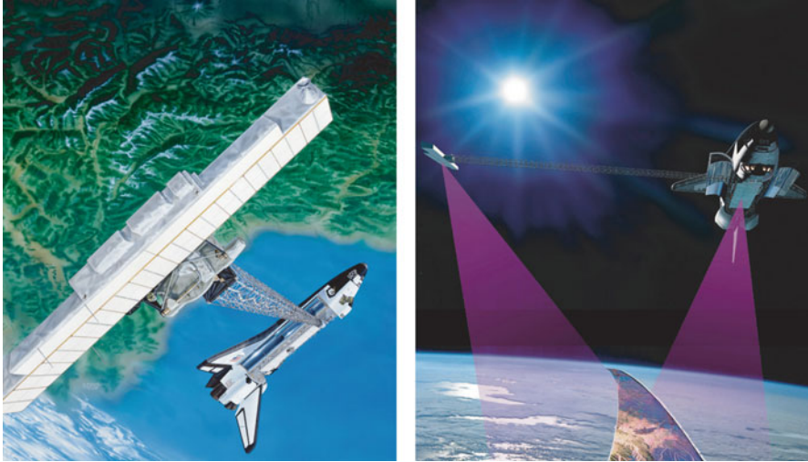
Fig. 12.26 The extended interferometric radar antenna on the SRTM shuttle (Credit: NASA/JPL-Caltech, Ball Aerospace & Technologies Corp.)
