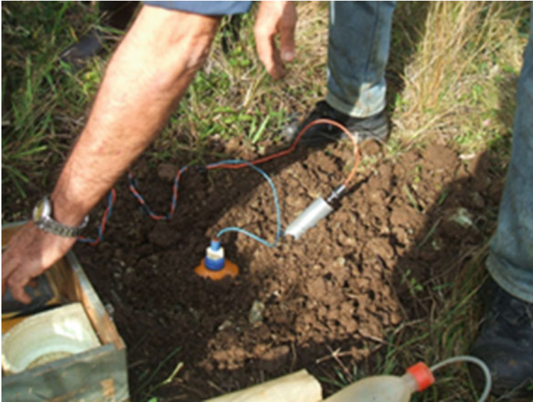
Fig. 2.1 Measurement of Redox Potential in soils
