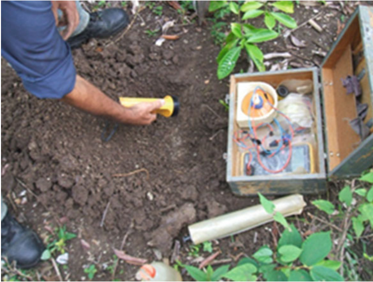
Fig. 2.2 Measurement of the Magnetic Susceptibility in soils
