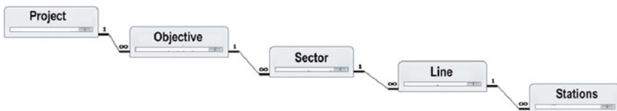
Fig. 4.2 Relationship of one to many of each of these fundamental entities of the system
