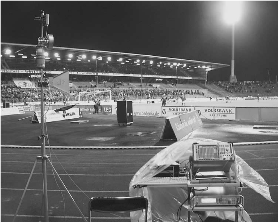
Figure 3.6 An example of the stadium tracking equipment set-up (antennae and computer) used by the Cairos match analysis system
