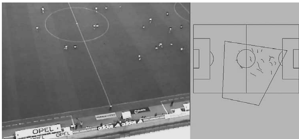
Figure 3.4 The pitch area covered by one particular camera using the AMISCO system (courtesy of Sport-Universal Process)
