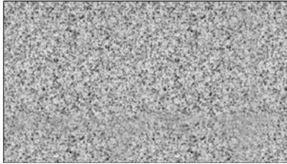
Fig. 10.12 Granular light patterns arise when light reflects from a diffuse or random scattering medium
