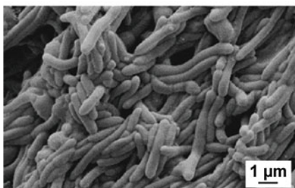
SEM of stainless surface from dairy industry
