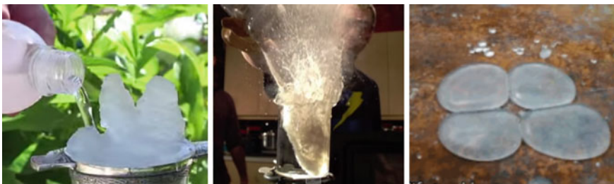
Fig. 8.12 Ice making from supercooled water [94] and superheated water exploding by adding sugar. The gel-like quasisolid water stays on a hydrophobic substrate. (public domain)
