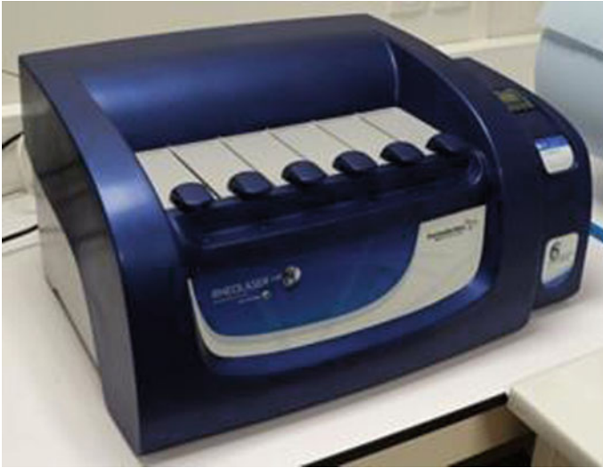
Fig. 2.9 Microrheology analyzer (Rheolaser LAB6™)
