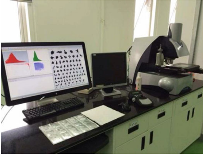
Fig. 2.10 Morphologi G3 optical microscope
