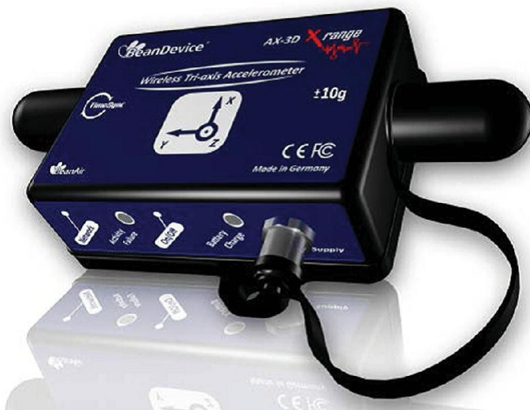
Figure 2.12 Wireless sensors for structural monitoring.
