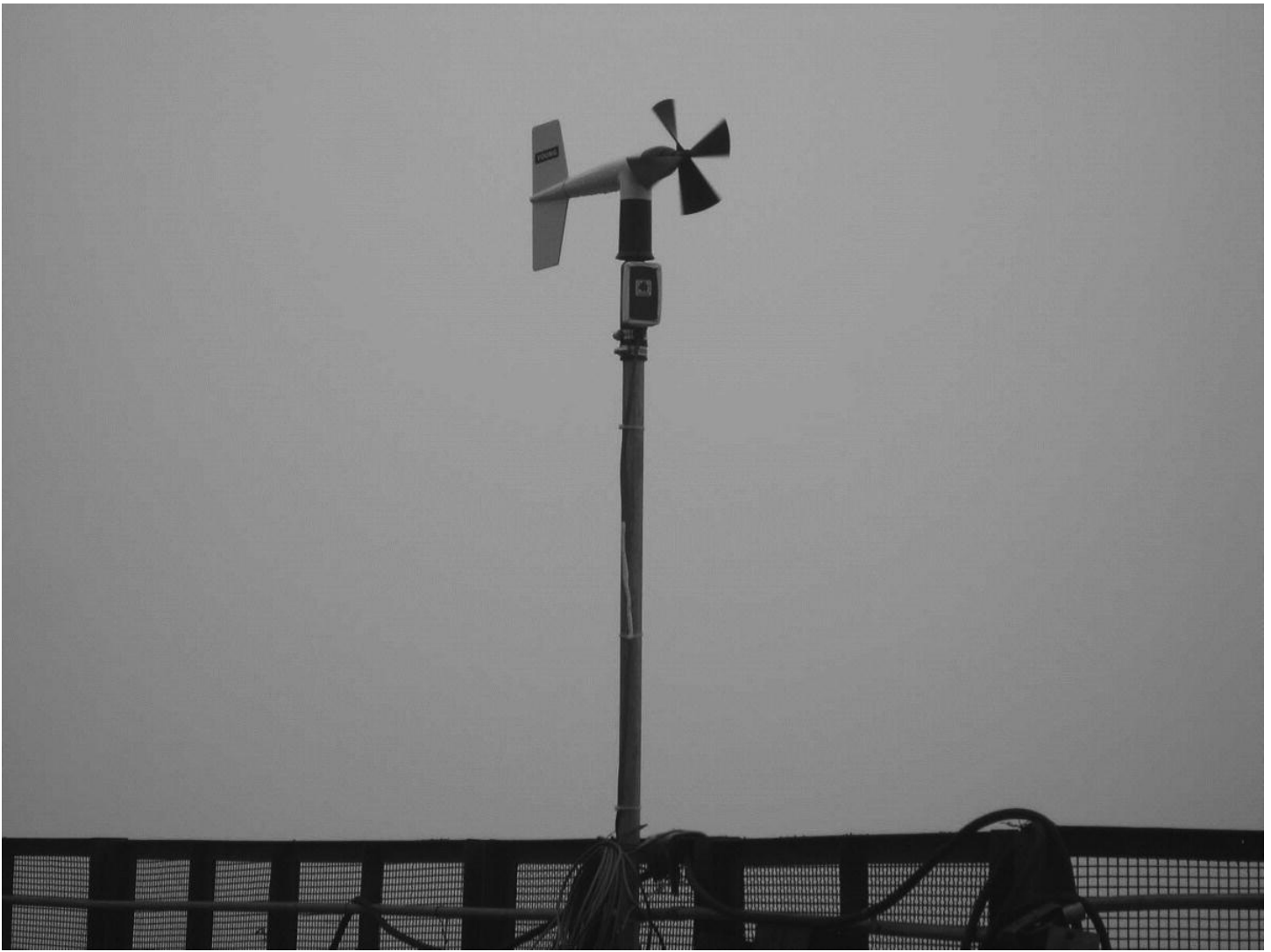
Figure 2.5 Anemometer (R.M. Young Model 05103L) installed on Canton Tower.
