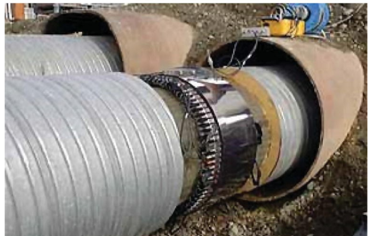
Figure 4.2 Equipment and applications of the guided wave technique.
