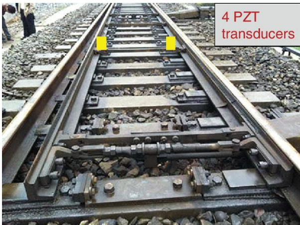
Figure 10.20 Undamaged rail turnouts and arrangement of PZT transducers on railway switch area.
