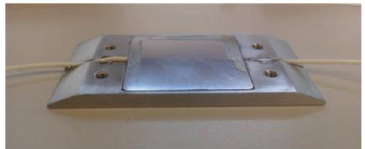
(b) The stainless steel packed water pressure sensor
