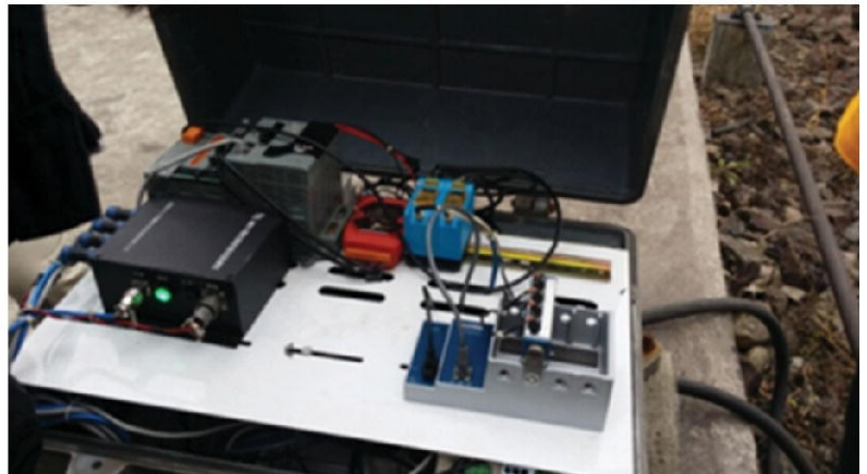
Figure 10.19 Piezoelectric (PZT) based acoustic emission sensing system for damage detection of rail turnouts.
