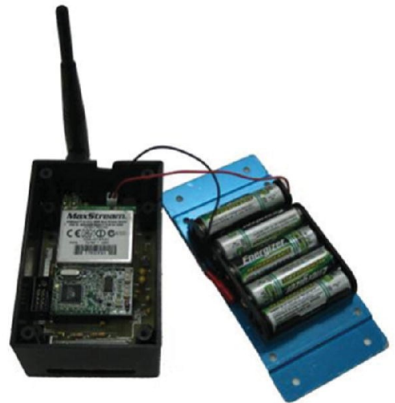
(b) Academic wireless sensing prototype (after Ni et al. 2011).
