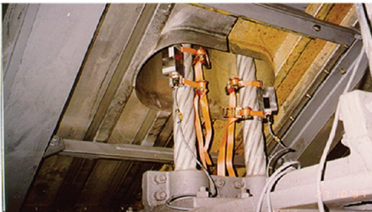
Figure 2.2 Accelerometers used in vibration monitoring of civil engineering structures.
