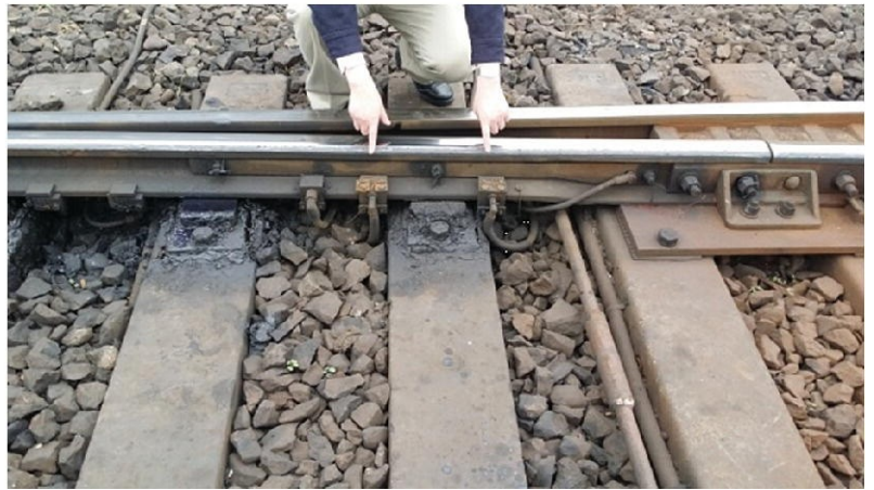
Figure 10.20 Undamaged rail turnouts and arrangement of PZT transducers on railway switch area.
