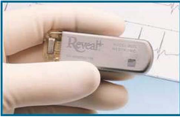
Fig. 17.16 The Reveal™, an implantable ECG loop recorder, is manufactured by Medtronic, Inc. (Minneapolis, MN)
