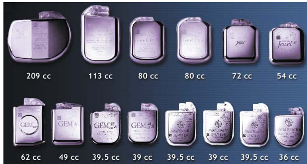
Fig. 27.18 The evolution of the implantable cardioverter defibrillator (ICD). Dramatic reductions in size have occurred, with simultaneous improvements in longevity, diagnostics, functionality, and memory
