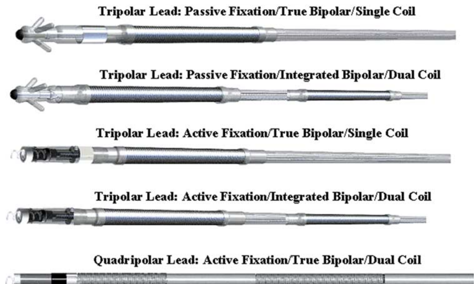
Fig. 27.40 Endocardial defibrillation leads. Various configurations are shown, including leads with active and passive fixation mechanisms, true and integrated bipolar pace/sense circuits, and/or single and dual defibrillation electrodes. The designs shown are typically placed in the right ventricle with the distal defibrillation coil within the right ventricular chamber and the proximal coil located in the superior vena cava
