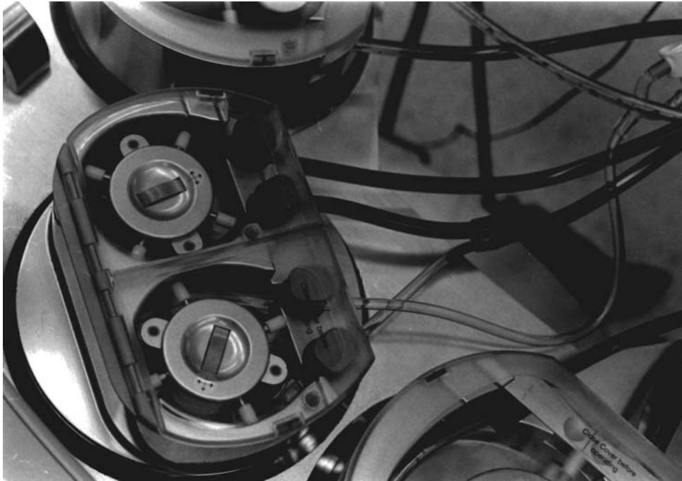
Fig. 30.7 Roller pumps of cardioplegia infusion system. The upper pump utilizes \frac{1}{4} in tubing to move the blood, and the lower pump runs crystalloid cardioplegic solution using \frac{1}{16} in tubing. The
