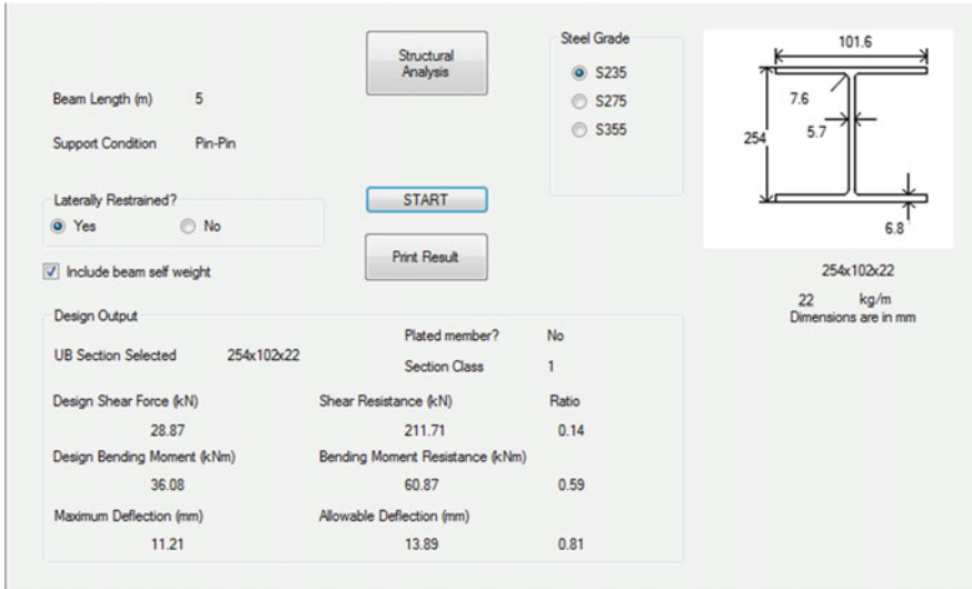
Fig. 2.4 Result for Example 2-1 using steel design based on EC3 program
