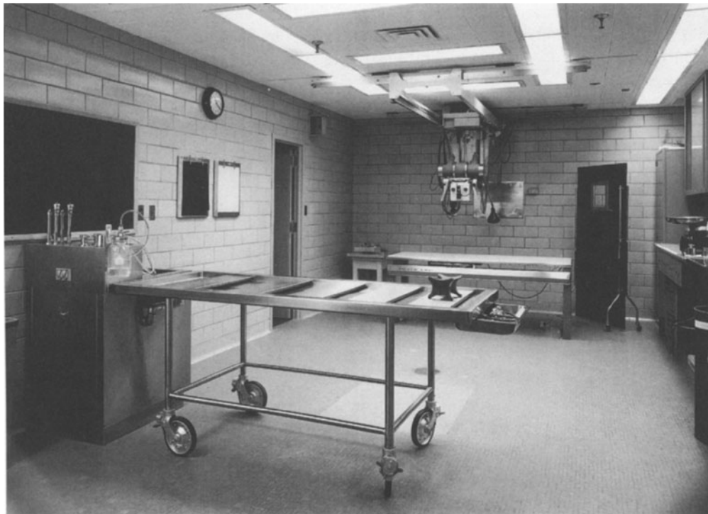
Fig. 10-2. Shielded autopsy room for roentgenologic examination. In the background is a Machlett Super Dynamax Tube and a Picker X-ray table. In adjacent room to the left, a 300-mA Keleket X-ray machine with a 125-kV generator is installed. In the foreground is a mobile autopsy table with a separate service island.
