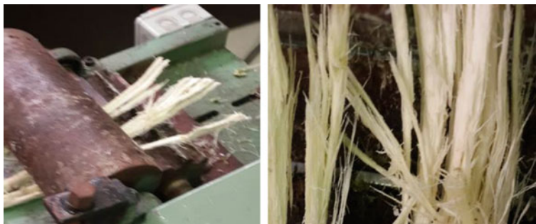
Fig. 1 Okra stem fiber extraction process and extracted okra stem fibers
