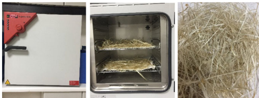
Fig. 2 Drying-oven, drying process of fibers and dried okra stem fibers
