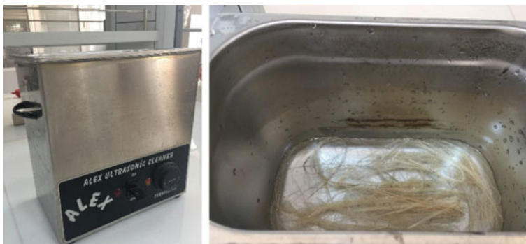
Fig. 6 Ultrasonic energy bath and processing of the okra stem fibers for the ultrasonic energy method
