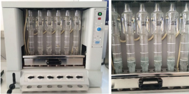
Fig. 11 Cellulose determination instrument and processing of okra stem fibers
