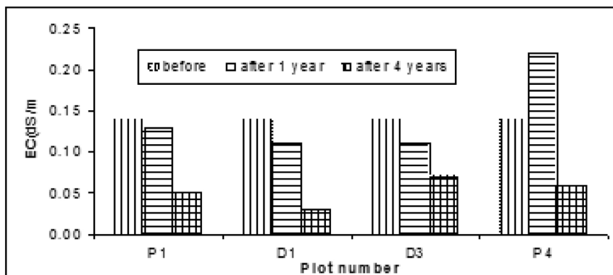
FIGURE 9.13b Change of soil EC (dS/m) over time in bio-drainage plantation.
