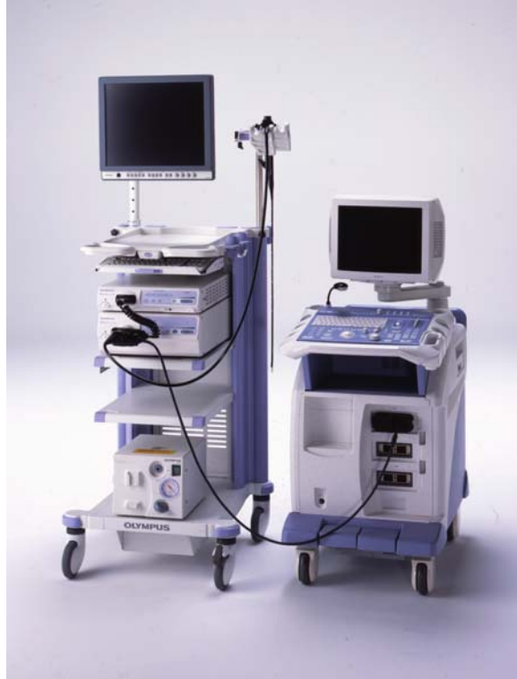
Fig. 8.15. The high-end ultrasound scanner (Aloka alpha 5, Tokyo, Japan) in combination with the convex probe endobronchial ultrasound.
