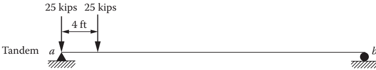
FIGURE 3.39 Design tandem load position for shear at support.
