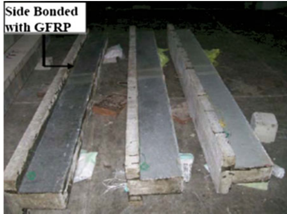
Fig. 3.9 Details of strengthening schemes with side-bonded GFRP
