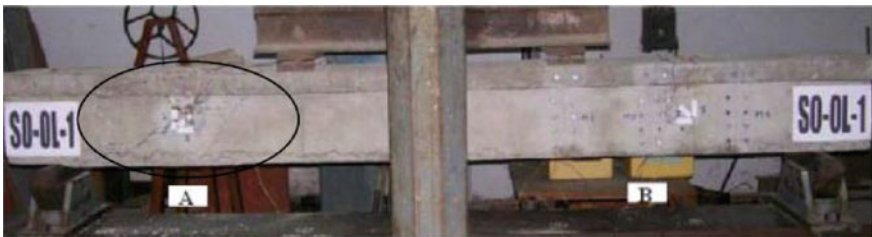
(a) Cracking Pattern of Full Beam Specimen
