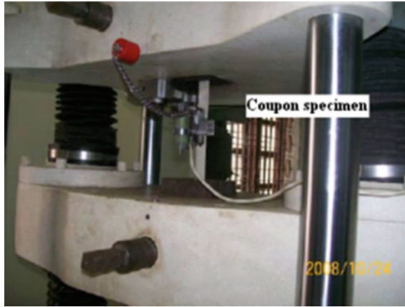
Fig. 3.13 UTM showing the coupon specimen
