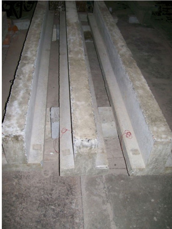
Fig. 3.7 RC T-beams after curing
