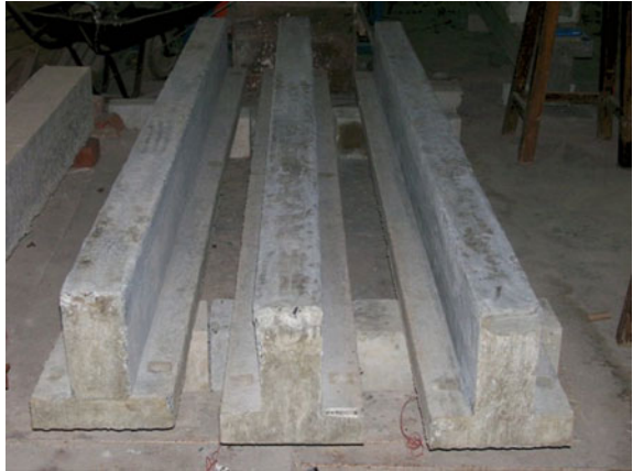
Fig. 3.3 Specimens before applying GFRP
