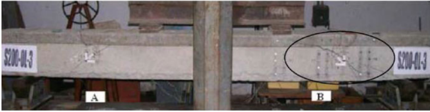
(a) Cracking Pattern of Full Beam Specimen
