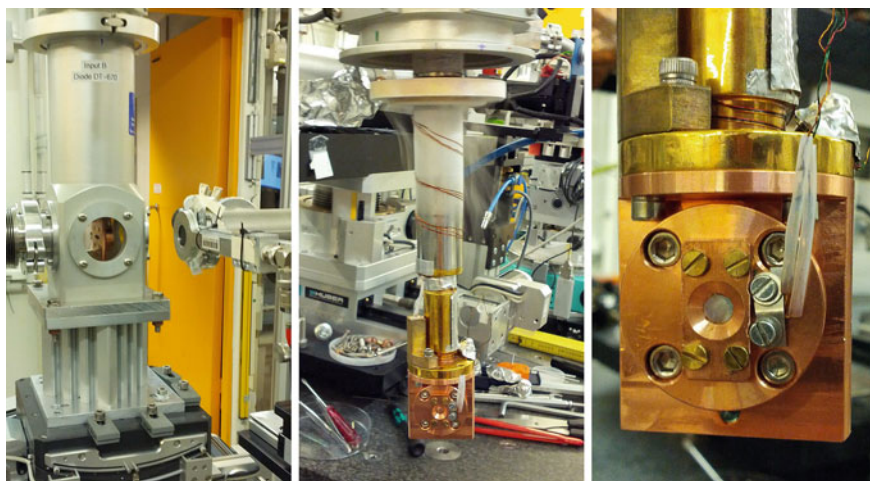
Fig. A.6 Cryostat at PETRA III. Left Closed cryostat with mounted sample. Middle Cryostat cold finger removed for sample switching. Right Close-up view of sample mounted on cryostat cold finger
