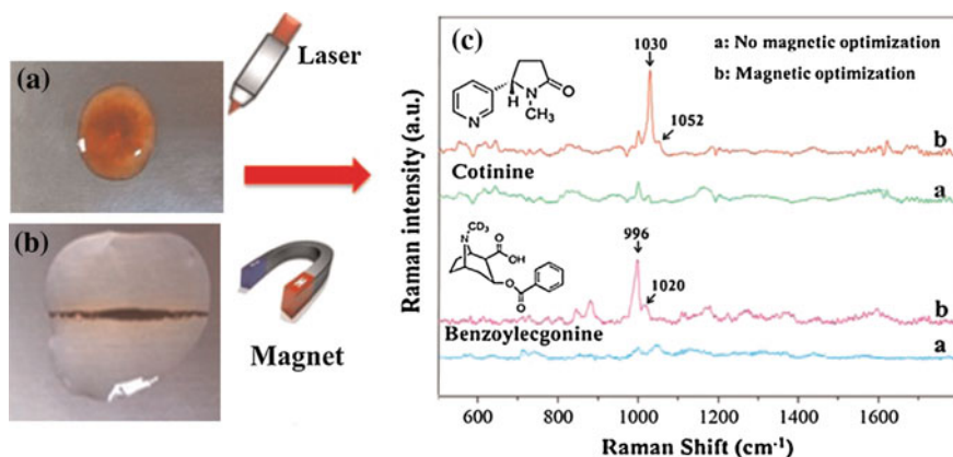
Fig. 4.5 Scheme for the procedure of detection of drug-related biomarkers in saliva with magnetically optimized SERS protocol. a Saliva containing drug mixed with MNPs onto aluminium foil. b MNPs were accumulated in small spot using a magnet. c SERS spectra of cotinine and benzoylecgonine obtained with and without magnetic optimization. Inset chemical structures of both compounds (adapted with permission from Yang et al. 2015. Copyright 2015 Elsevier B.V.)
