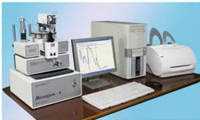
Fig. 3.21 “Milichrom-6 Leader” liquid microcolumn chromatograph. Photo taken from an advertising brochure
