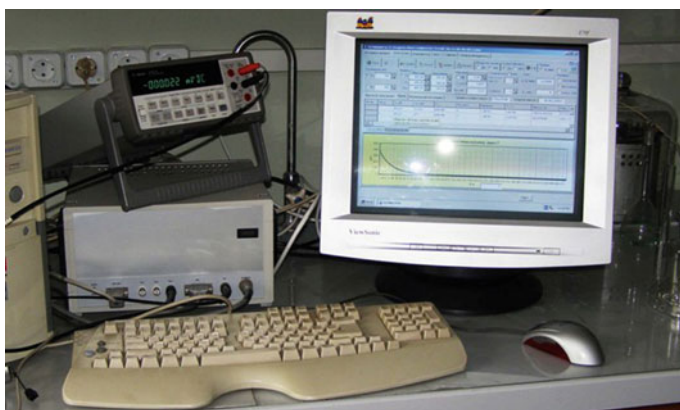
Fig. 4.8 Precision coulometer, PIK-200, developed at the V. I. Vernadskii Institute of Geochemistry and Analytical Chemistry of the USSR Academy of Sciences. Photo taken from the website of the Vernadskii Institute of Geochemistry and Analytical Chemistry
