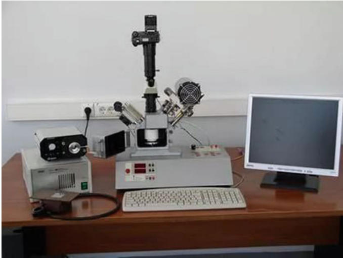
Fig. 1.11 “Focus-M” microanalyzer with Kumakhov X-ray lens. Figure provided by the Institute of X-Ray Optics
