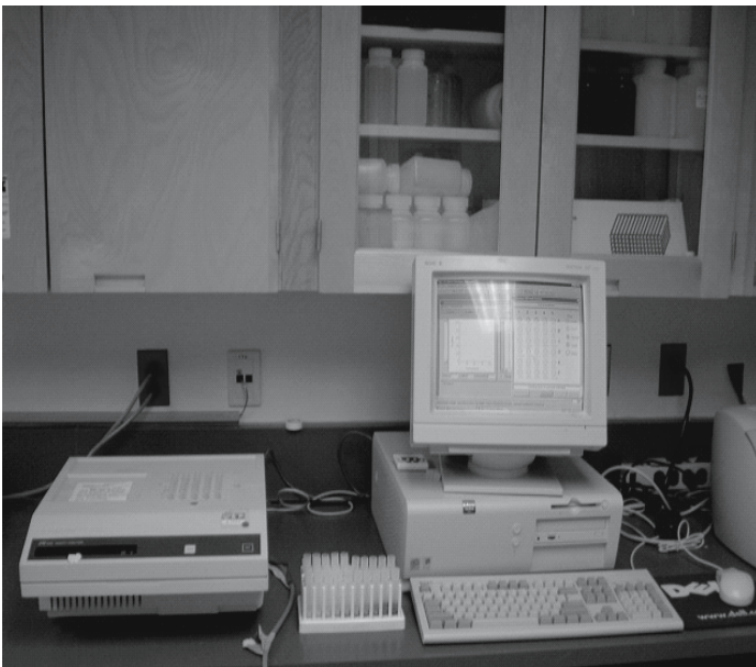
Figure 2. M500 Microtox photometer, solid-phase tubes, and the computer to run the test, calculate the endpoints, and store the data.
