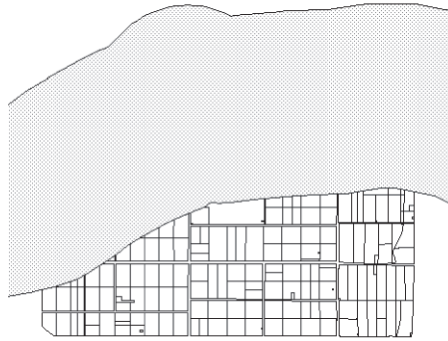
FIGURE 3.8. Land parcels outside the river buffer have been excluded from consideration, because they are too great a distance from the river for effluent discharge.
