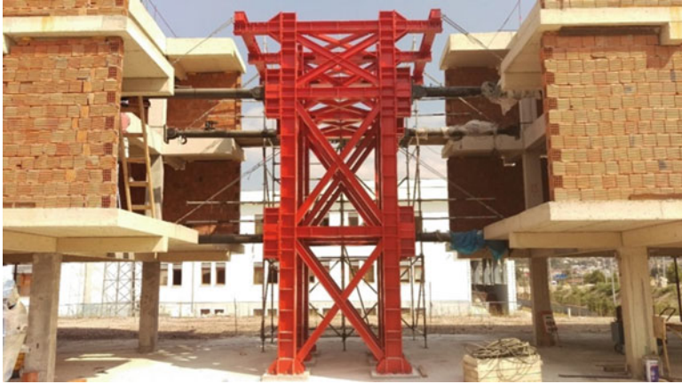
Fig. 22.7 Reaction frame and loading system (Tore et al. 2017)
