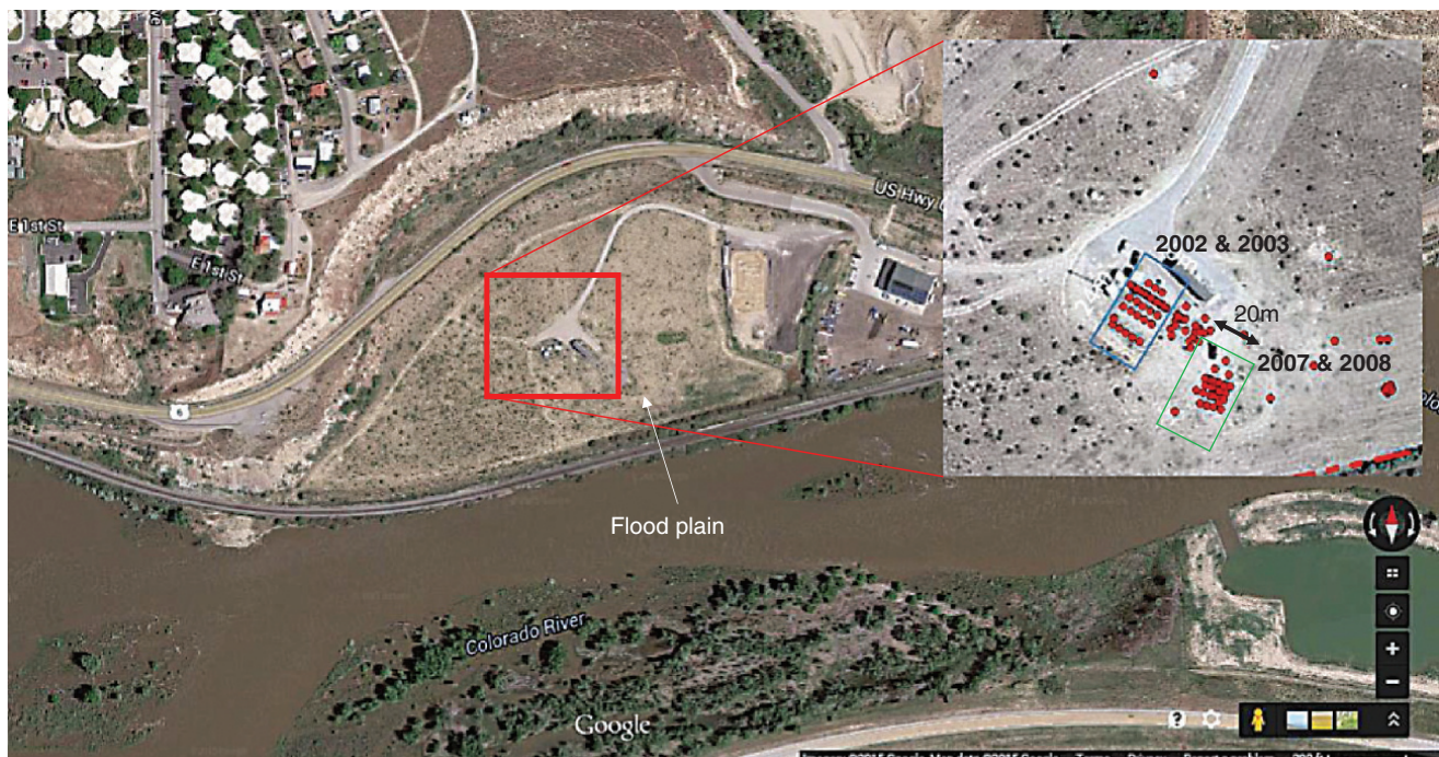
Figure 1.10 Rifle site with locations of the four uranium bioremediation experiments conducted in the years 2002, 2003, 2007, and 2008. The areal extent of 2007 and 2008 experiments are approximately 20 m × 20 m. The terrain map is obtained from Google Earth. Location of the wells (indicated by the red dots) for different years are referred from Yabusaki et al. [2007].
