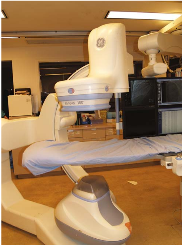
Fig. 2. An x-ray system with digital flat-panel technology.
