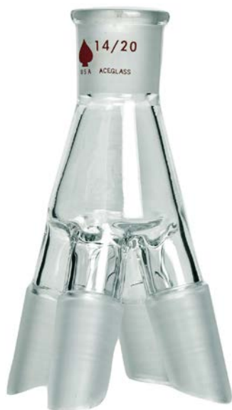
Figure 3.2 A cow adapter for vacuum distillation with collection of several fractions.
