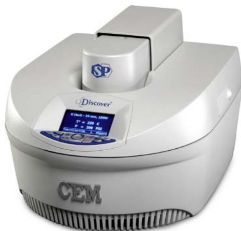
Figure 6.5 A microwave reactor for use in organic synthesis.
