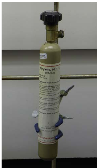
Figure 4.1 Lecture bottles used to hold and deliver small quantities of reagent gases.
