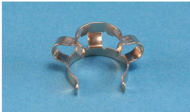
Figure 5.6 Metal clip for a ground-glass joint. Photo courtesy of Kimble/Kontes.
