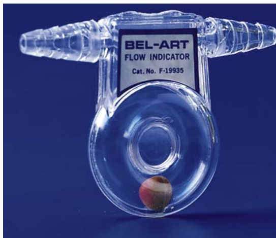
Figure 5.22 A flow indicator for insertion into tubing that delivers cooling water to a condenser. The ball circles the device when water is flowing through the tubing. Bel-Art SP Scientific.
