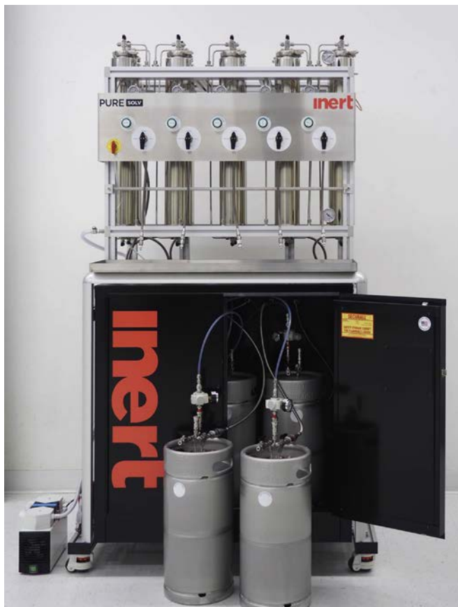
Figure 7.4 A “Grubbs” solvent purification system. Photo provided by Inert.
