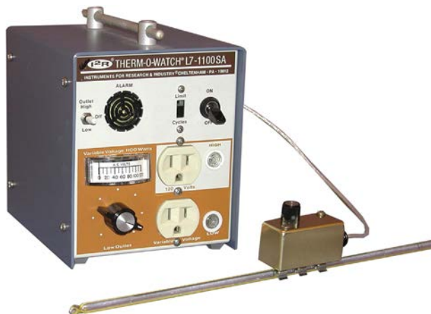
Figure 6.4 A THERM-O-WATCH monitors the temperature via a sensor placed on a mercury thermometer and controls the power being delivered to a heating device to maintain a constant temperature. Similar sensors are available to ensure water is flowing before heat is applied to a system that requires cooling.
