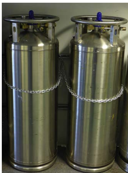
Figure 6.8 Large dewars for storage of liquid nitrogen. These tanks are around 1.5 m in height.
