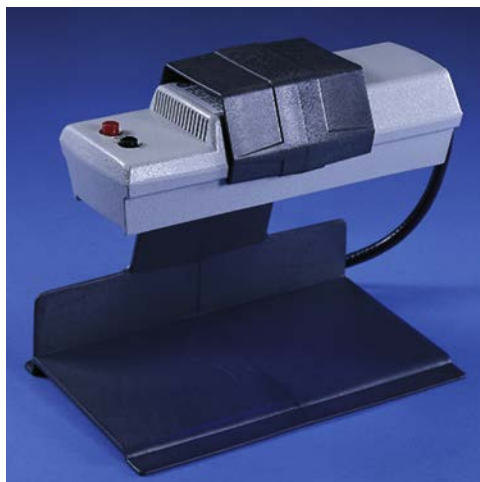
Figure 10.9 A long-wavelength UV lamp used for initial visualization of thin layer chromatography plates. Photo provided by UVP LLC.
