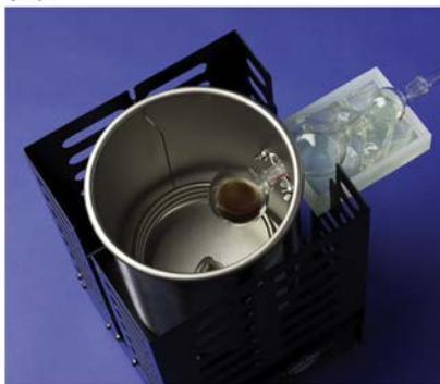
Figure 14.2 A Kugelrohr distillation oven. (A) Side view; (B) top view. © Sigma-Aldrich Co. LLC.
