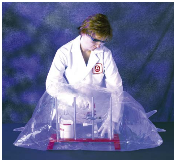
Figure 5.7 This mid-sized glove bag is 39×48 in and has a 22 in diameter opening to load equipment.
