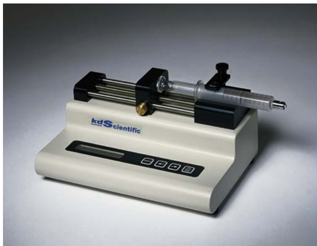
Figure 5.16 A syringe pump accepts a variety of sizes of syringes and drives a ram against the plunger at a constant rate. The rate of liquid delivery is variable based on the size of the syringe and the setting of the syringe pump.
