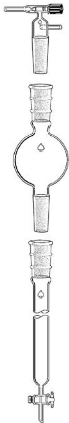
Figure 14.3 A flash chromatography column, reservoir, and air control valve.
