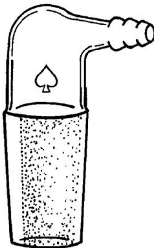
Figure 5.10 A gas inlet that can be used to attach a flask to the inert atmosphere manifold.
