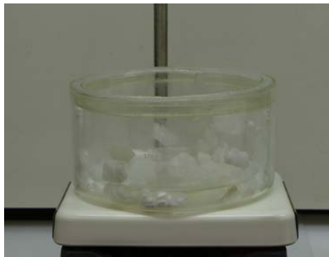
Figure 6.6 A homemade insulated cold bath.
