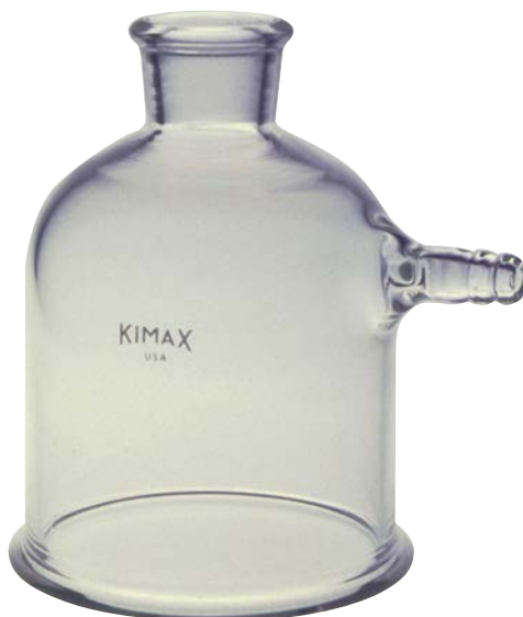
Figure 10.1 A filtering bell jar can be used to apply vacuum to a spotted thin layer chromatography plate to remove poorly volatile reaction solvents. Photograph provided by Kimble/Kontes.
