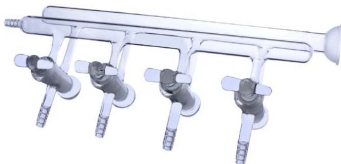
Figure 5.12 (A) A simple manifold to deliver inert gas to several vessels. (B) A double manifold that can deliver inert gas and apply vacuum.
