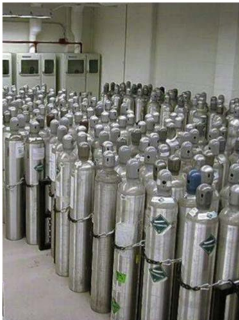
Figure 4.3 Large gas cylinders typically used for gases such as He, N 2 , and H 2 . Photo provided by Airgas, Inc.
