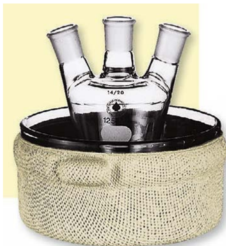
Figure 6.3 An oil bath with an integral heating element.
