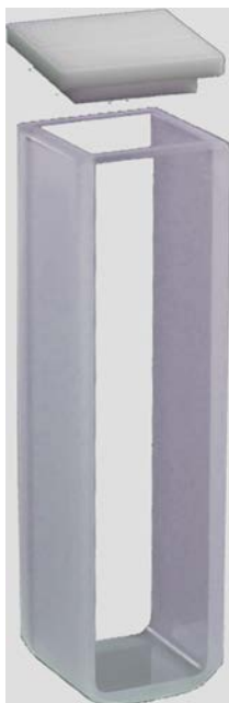
Figure 15.3 A quartz UV cuvette with Teflon cap.
