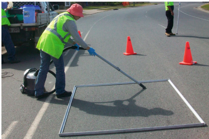
Fig. 2.5 Road build-up sampling
