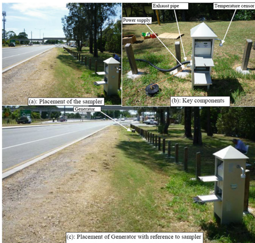
Fig. 2.2 Air sampling in the field
