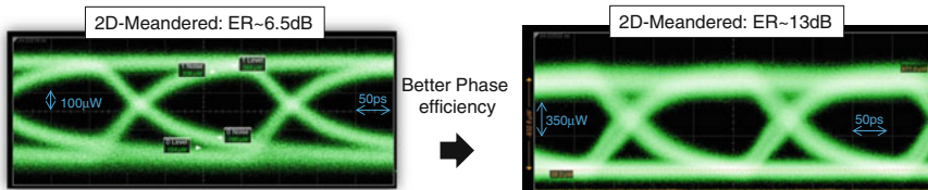
Fig. 10.18 Measured eye diagrams at the wafer level of a meandered multisection modulator based on the optimized doping and junction offset position for a maximum modulation efficiency
