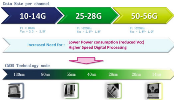
Fig. 10.3 Correspondence between photonics nodes and CMOS nodes
