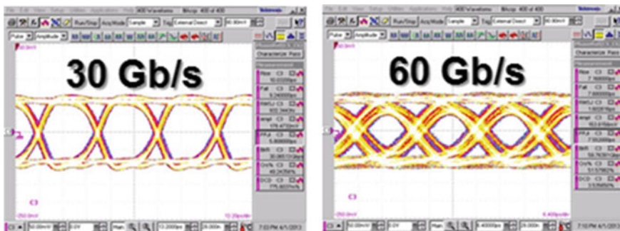
Fig. 13.11 Eye diagrams of a heterogeneously integrated photodetector integrated with SiGe driver circuit, operating at 30 and 60 Gb/s [5]
