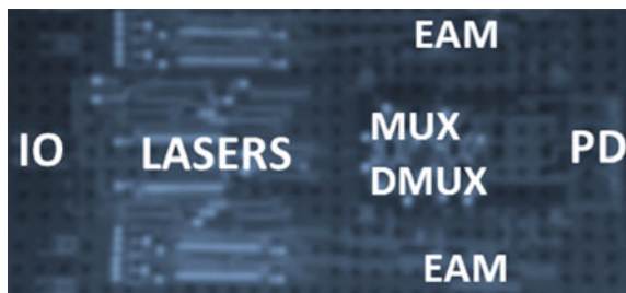
Fig. 13.16 Photograph of a 4 \times 25 Gb/s transceiver PIC developed by Aurion that integrates lasers, modulators, a multiplexer, a demultiplexer, photodiodes, and optical fiber coupler devices on a single silicon chip
