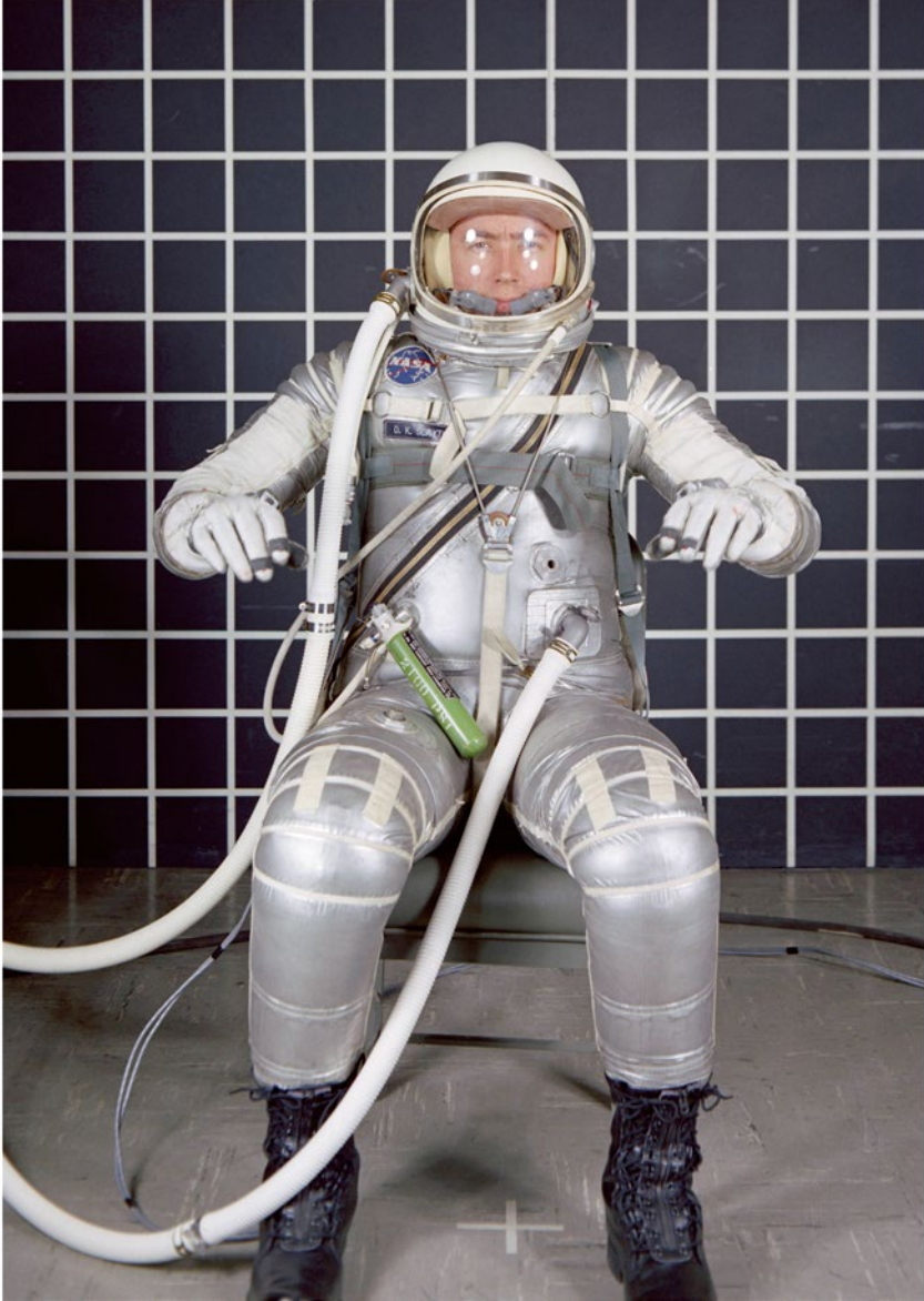
A suit technician wearing Deke Slayton's fully pressurized Mk. IV space suit during a mobility demonstration. (Photo: B. F. Goodrich)
