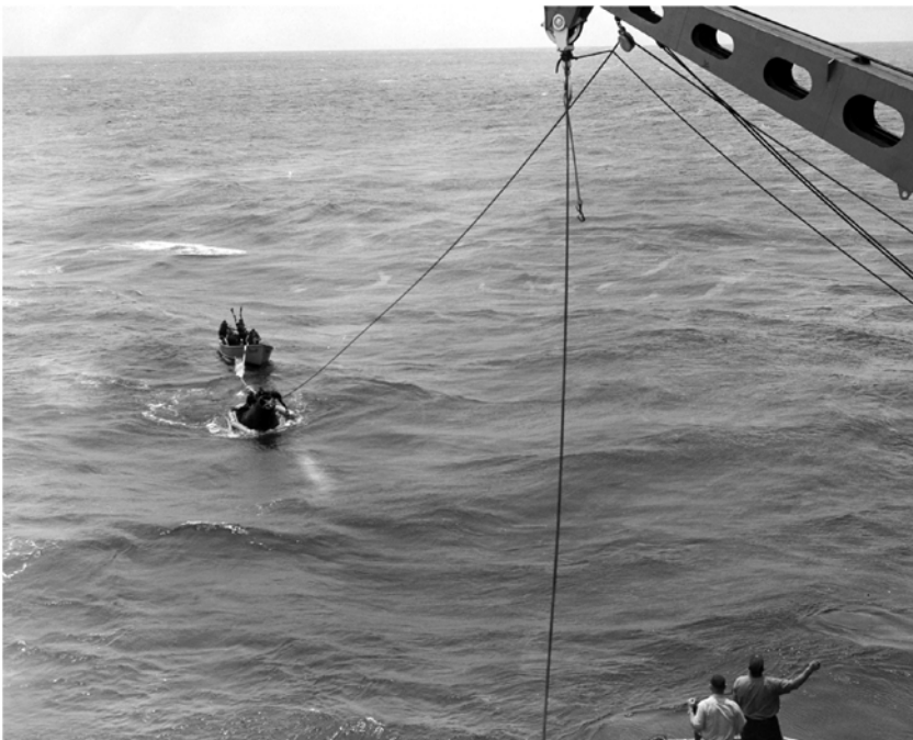
The whaleboat crew attaches the nylon tow rope to Sigma 7 , which is then slowly hauled towards the carrier as the boat stands by. (Photos: NASA)
