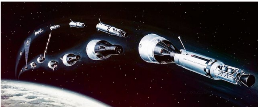
The mission profile for the Gemini VI rendezvous and link-up with the Agena target vehicle. (Photo: NASA)
