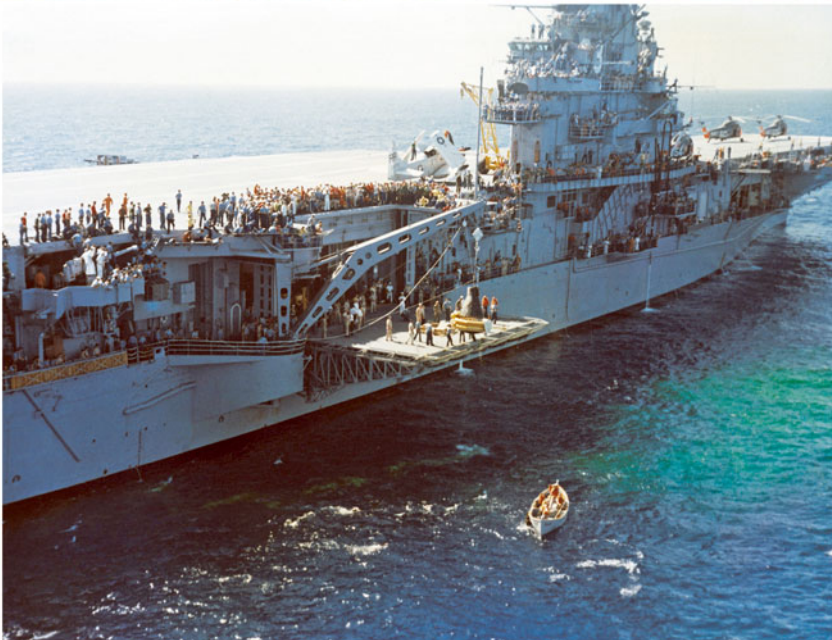
Sigma 7 is hoisted out of the water by boat crane, ready to be placed on a special pallet on the carrier's number 3 elevator. Note the ship's company crowding to one side of USS Kearsarge . (Photos: NASA)
