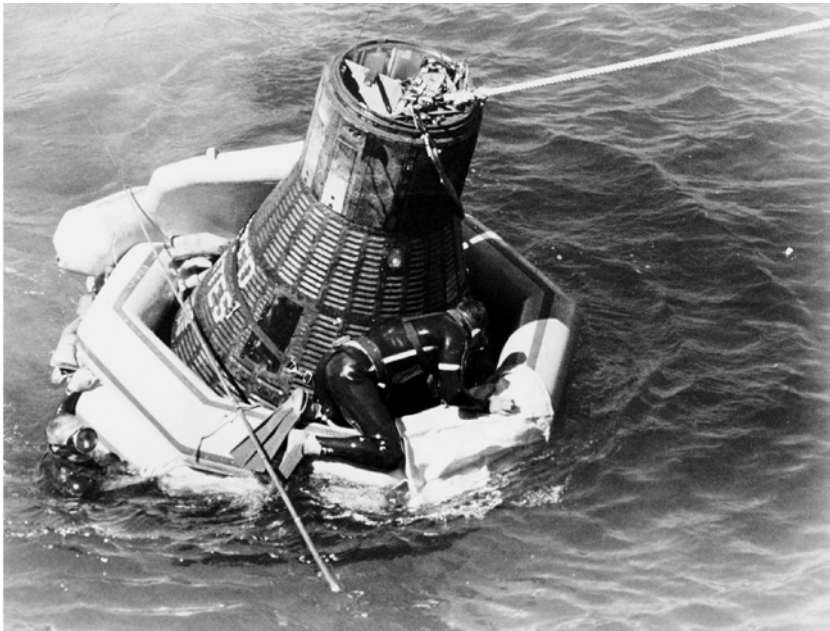
The Navy frogmen were dropped 15 feet into the water beside the bobbing spacecraft, and quickly installed the Stullken inflatable collar around Sigma 7 . (Photo: NASA)
