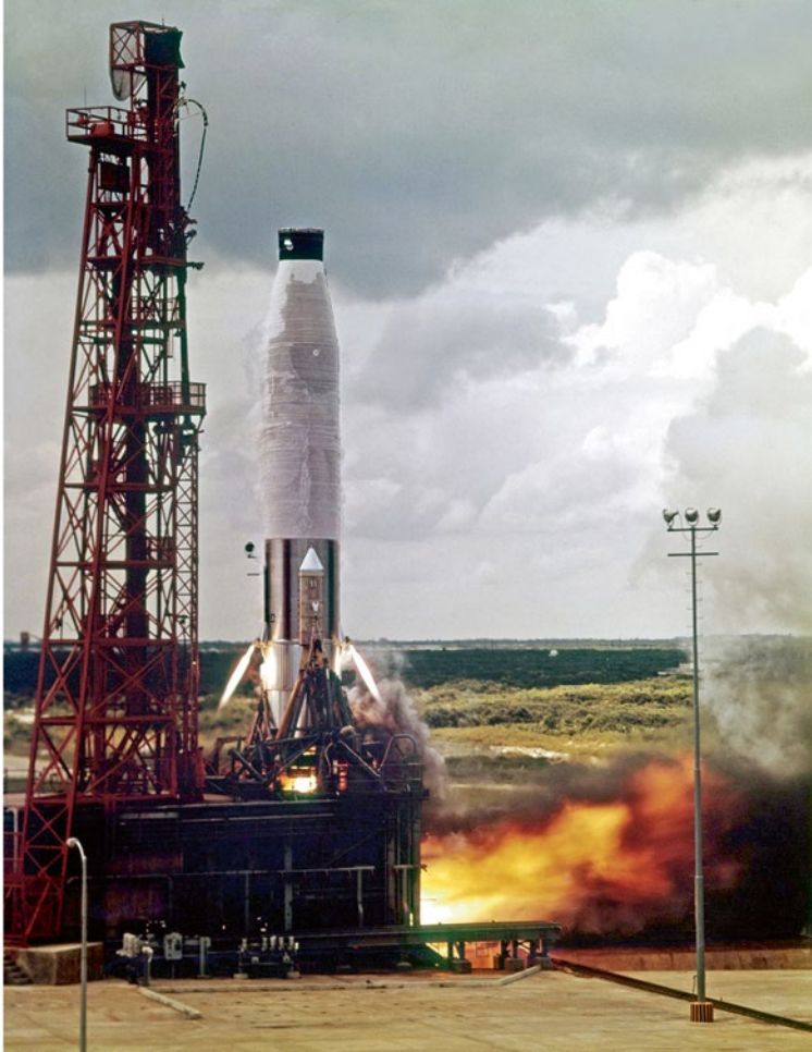
Prior to the installation of Sigma 7 atop Atlas 113-D, the rocket underwent a planned static test firing on Pad 14 to evaluate recent modifications. (Photo: NASA)
