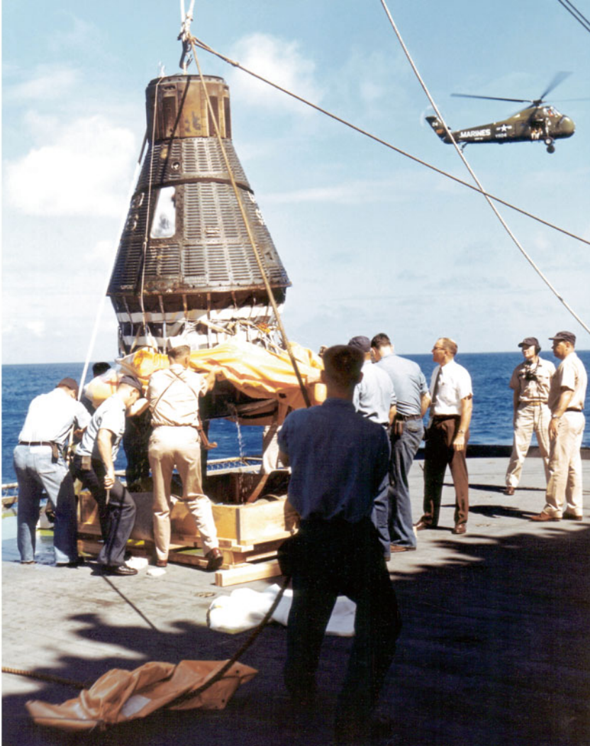
The Stullken collar, its job done, is punctured before the spacecraft can be lowered onto the pallet. (Photo: NASA)
