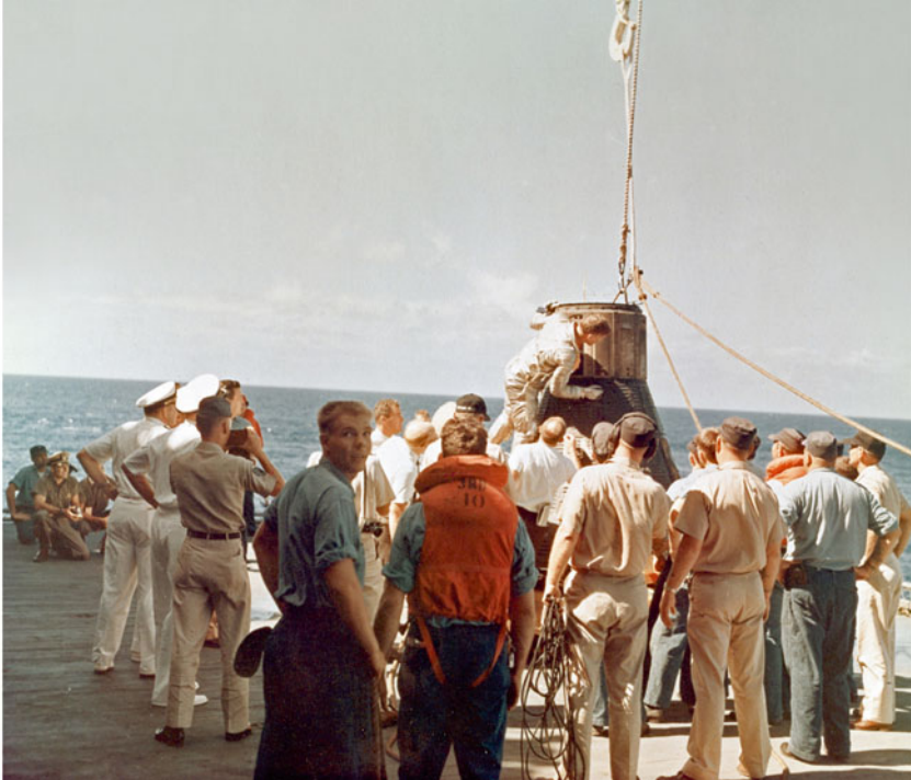
The astronaut climbs to the top of his spacecraft to check on the condition of the ablative shingles. (Photos: NASA)
