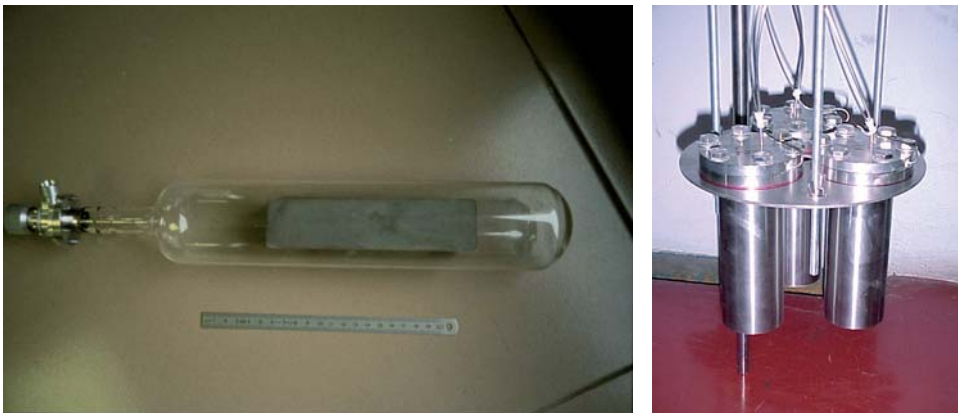
Figure 8 : Radiolysis experiments on cement pastes leading to know the total pressure and the composition of gases according to the duration of gamma irradiation : a) sealed glass phial around a test-bar 4 \times 4 \times 16 cm ; b) mini-containers out of stainless of 500\text{ cm}^3 (allowing a quasi-integral filling of cement paste) with outlets for P(H_2) measurement in line.
