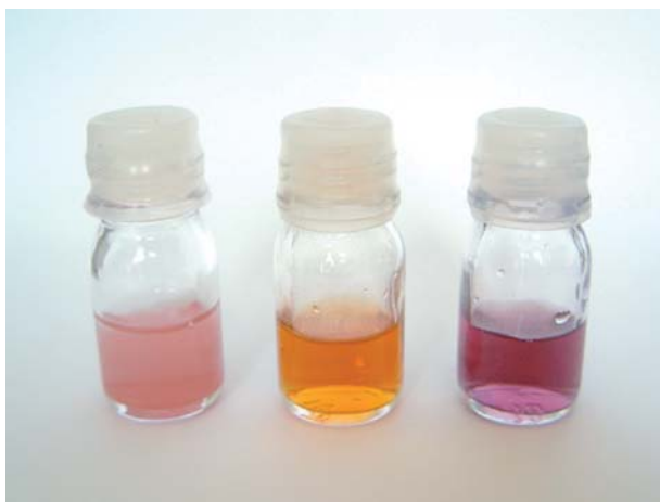
Figure 4 : Nanoclusters synthesized by irradiation of water solutions and stabilized by PVA. From left to right: copper, silver, and gold clusters. The colors of ultradivided metals are known from long. In the Middle Ages, they were produced in fused glasses under reducing conditions to produce stained glasses.
