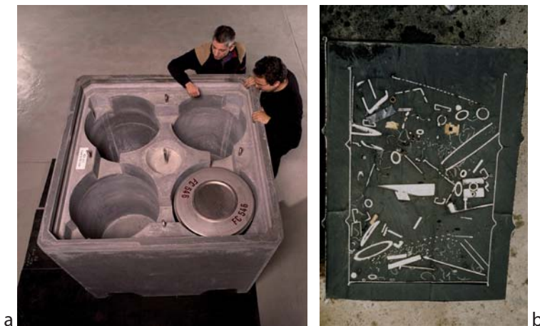
Figure 1 : Examples of cement-based matrices used in the conditioning of radioactive wastes : a) concrete container accommodating 4 primary waste forms ; b) mortar for embedding metallic wastes.
