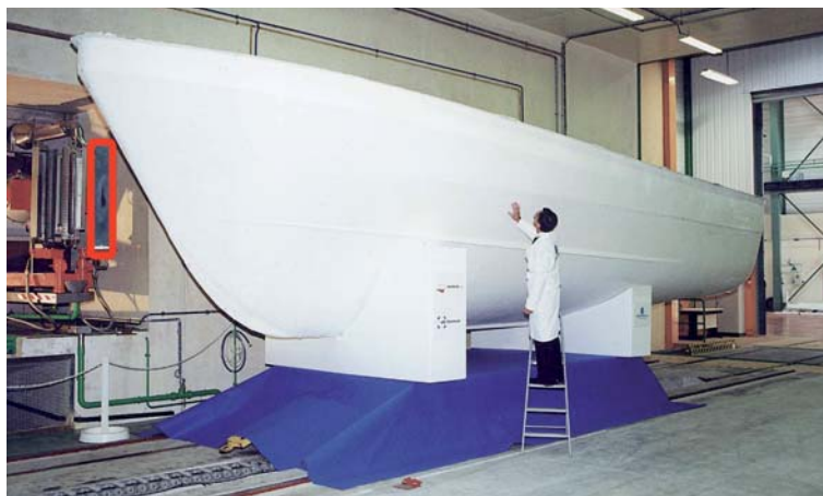
Figure 7 : Glass/polyester 10 meter-long ship hull cured by EB and X-ray induced polymerization. EB gun is circled by red line. (Courtesy of Intermarine and Astrium Space Transportation.)
