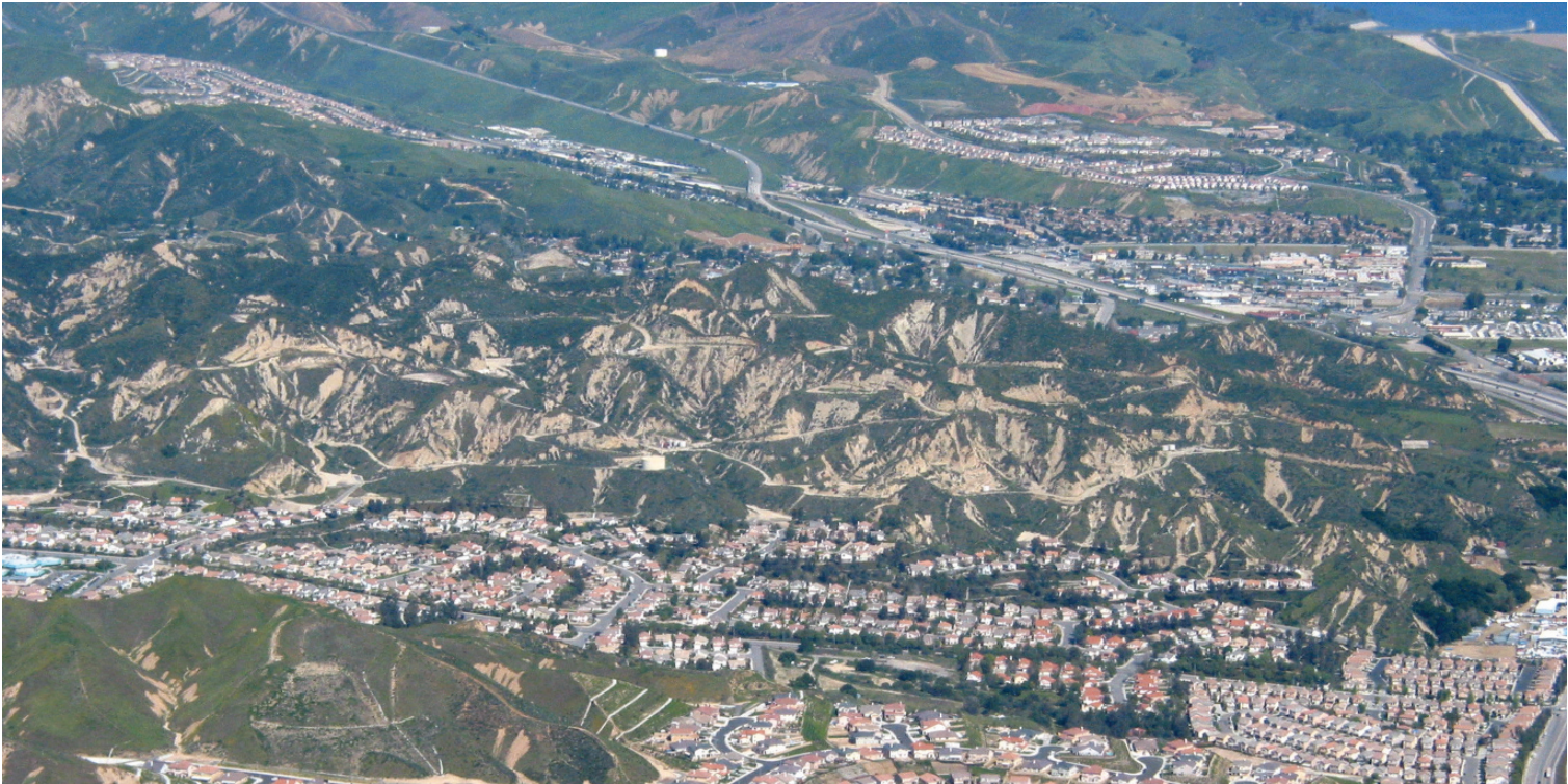
Figure 1.10 Photograph showing abundant shallow landslides and debris flows near Valencia, Los Angeles County, California. The light, un-vegetated scars are shallow failures of hillslope material caused by heavy rainfall during the winter of 2005 (photo by the authors).
